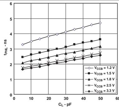
Figure 6. Typical A-to-B Propagation Delay, High to Low
