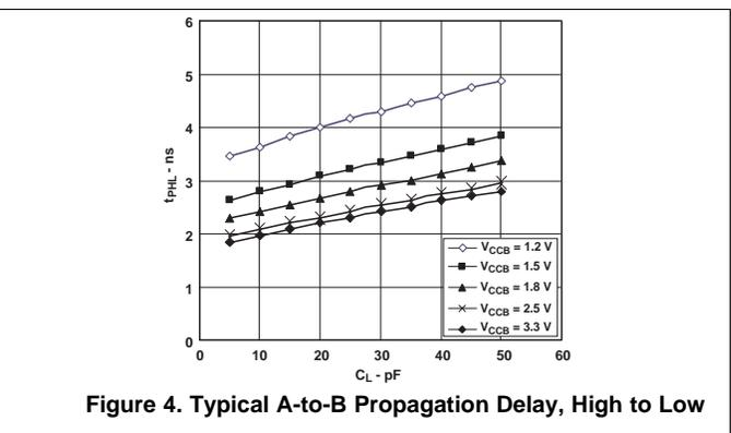
Figure 4. Typical A-to-B Propagation Delay, High to Low
