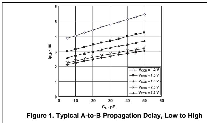
Figure 1. Typical A-to-B Propagation Delay, Low to High
