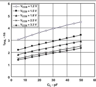
Figure 8. Typical A-to-B Propagation Delay, High to Low
