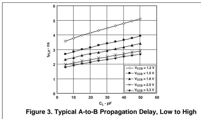
Figure 3. Typical A-to-B Propagation Delay, Low to High
