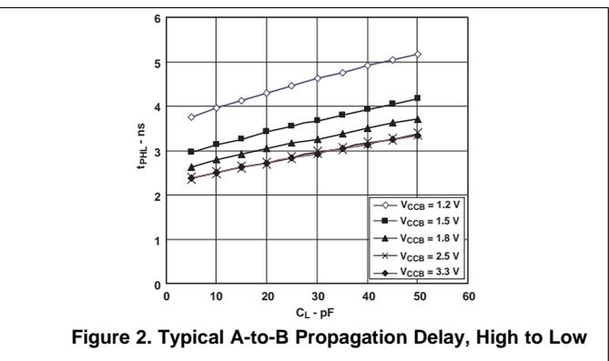
Figure 2. Typical A-to-B Propagation Delay, High to Low
