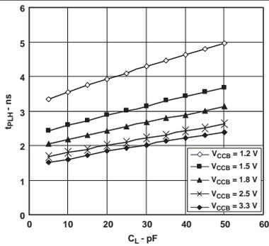
Figure 5. Typical A-to-B Propagation Delay, Low to High
