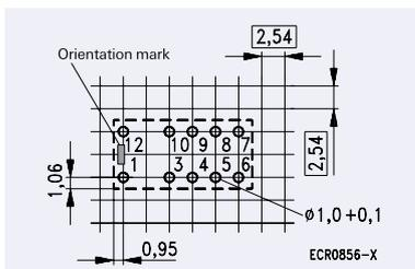
Note: Hole for pin 6 and 7 only for latching with 2 coils. Basic grid 2.54 mm
