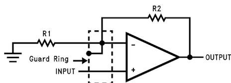
Figure 30. Non-Inverting Amplifier Guard Ring Connections
