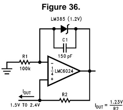
(Upper limit of output range dictated by input common-mode range; lower limit dictated by minimum current requirement of LM385.)
