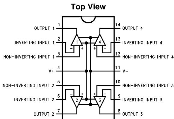
**Figure 1. 14-Pin DIP and SOIC Package**
