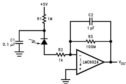
A 5V bias on the photodiode can cut its capacitance by a factor of 2 or 3, leading to improved response and lower noise. However, this bias on the photodiode will cause photodiode leakage (also known as its dark current).
