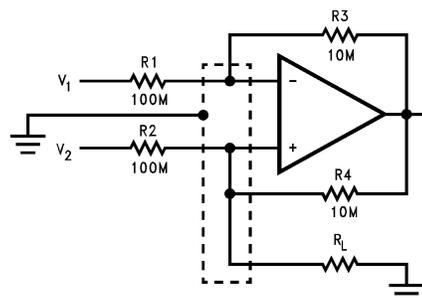
Figure 32. Howland Current Pump Guard Ring Connections
