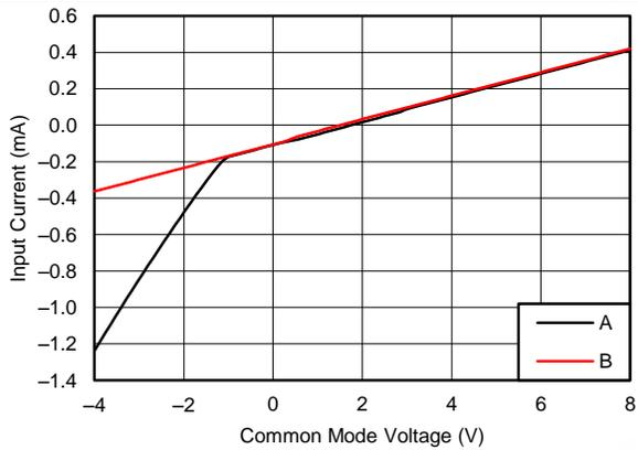
Figure 1. RS422 Port Current vs Common-Mode Voltage
