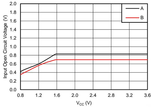
**Figure 20. RS422 Port Open-Circuit Voltage vs V<sub>CC</sub>**
