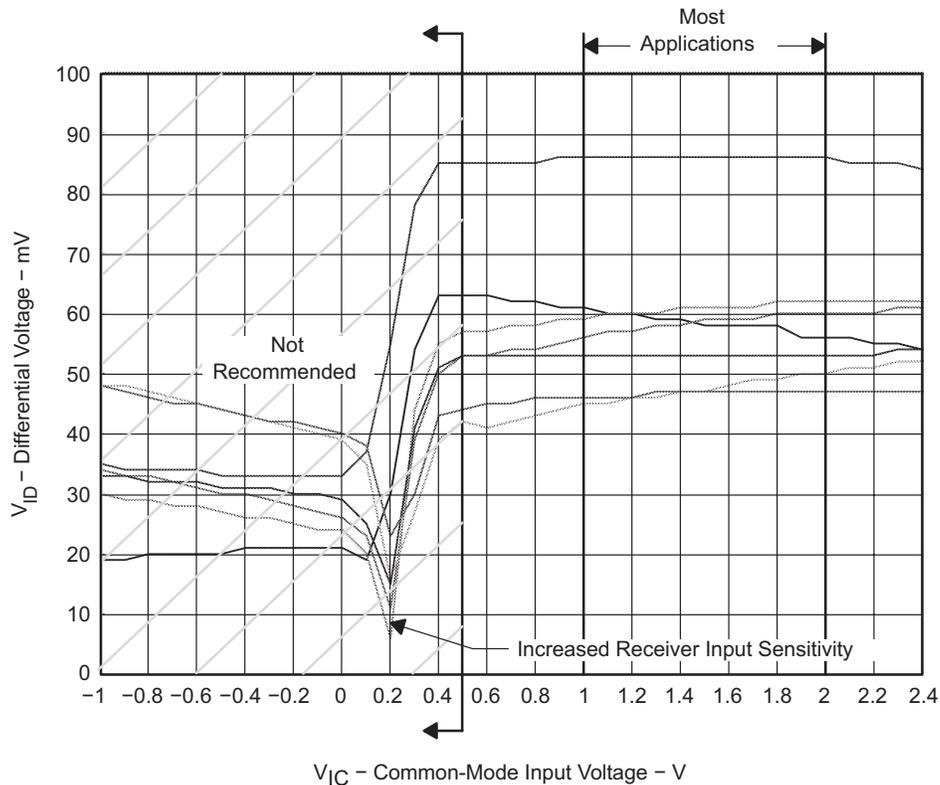
**Figure 13.  $V_{IC}$  vs  $V_{ID}$  Receiver Sensitivity Levels**
