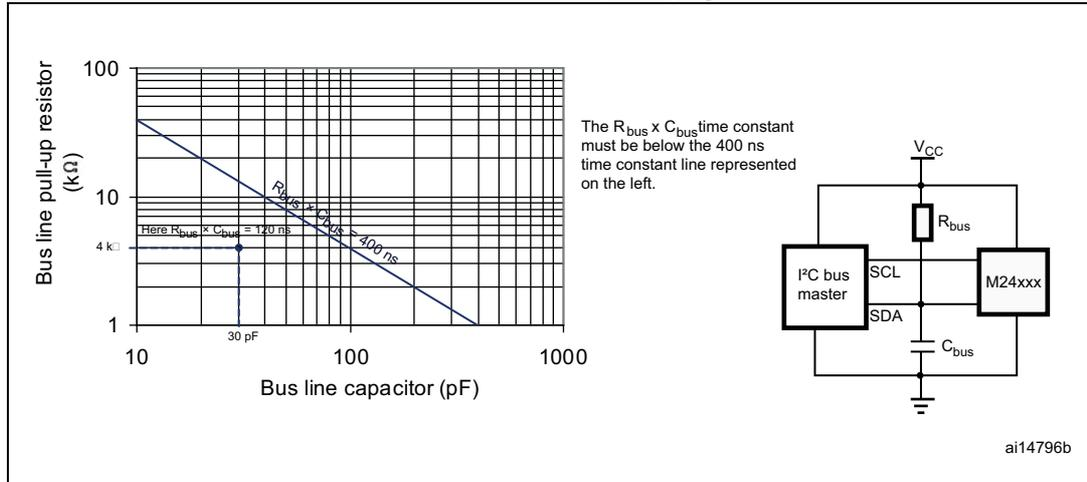
**Figure 13. Maximum  $R_{bus}$  value versus bus parasitic capacitance ( $C_{bus}$ ) for an I<sup>2</sup>C bus at maximum frequency  $f_C = 1$  MHz**
