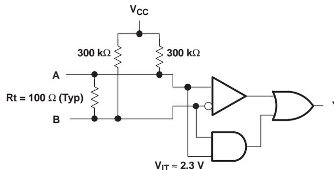
Figure 22. Open-Circuit Fail Safe of the LVDS Receiver
