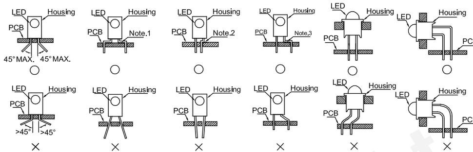
"○" Correct mounting method "×" Incorrect mounting method
