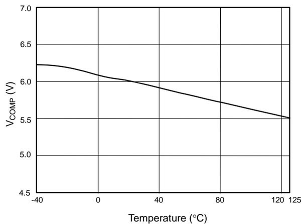
Fig. 11 V<sub>COMP</sub> open loop voltage vs. Temperature
