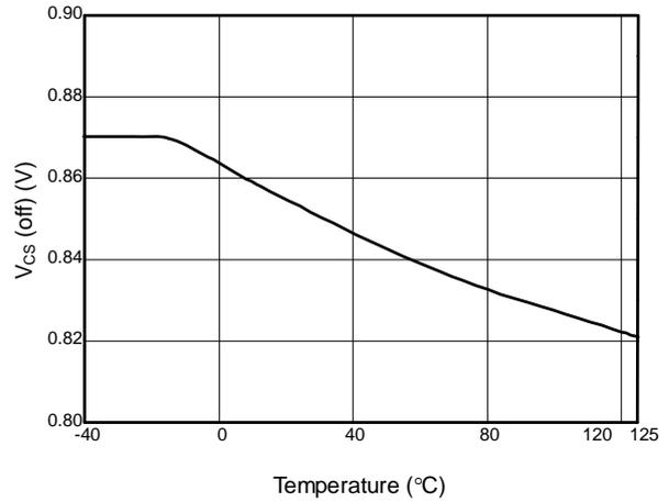
Fig. 8 V<sub>CS</sub> (off) vs. Temperature
