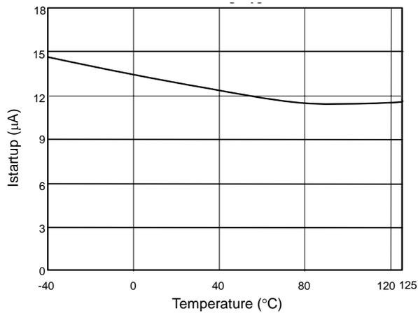
Fig. 9 Start up Current (I<sub>start up</sub>) vs. Temperature
