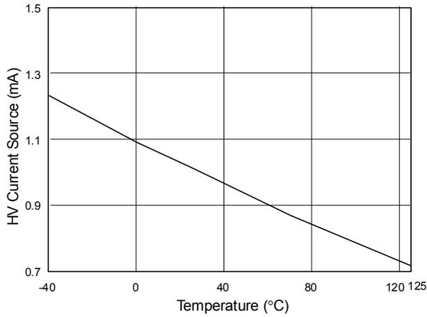
Fig. 1 HV Current Source vs. Temperature (HV=500V, Vcc=0V)
