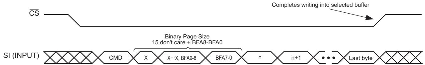
**Figure 20-3. Buffer to Main Memory Page Program (Data from Buffer Programmed into Flash Page)**
