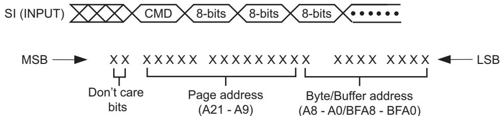
**Figure 19-4. Command Sequence for Read/Write Operations for a 528-Byte Page Size (Except Status Register Read, Manufacturer, and Device ID Read)**
