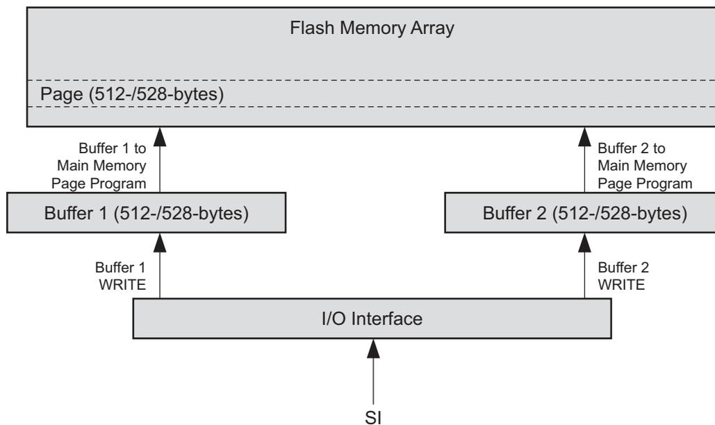
**Figure 20-2. Buffer Write**
