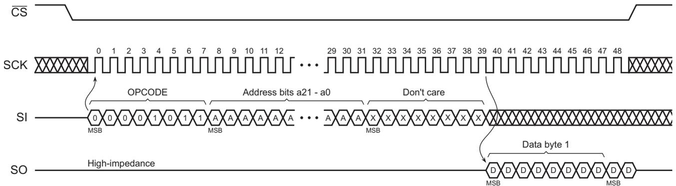
Figure 22-3. Continuous Array Read (Low Frequency: Opcode 03H)
