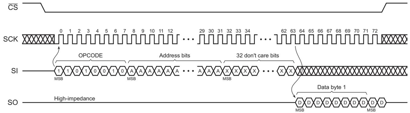
**Figure 22-5. Buffer Read (Opcode D4H or D6H)**
