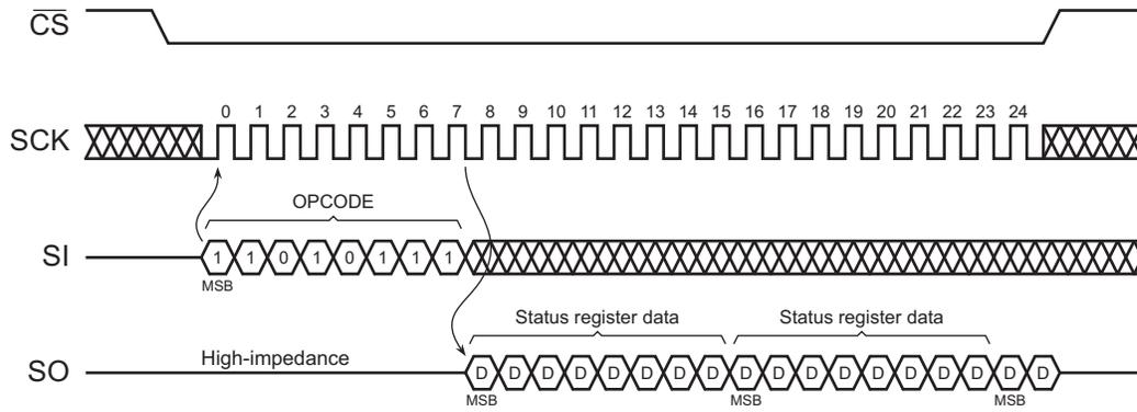
**Figure 22-11. Manufacturer and Device Read (Opcode 9FH)**
