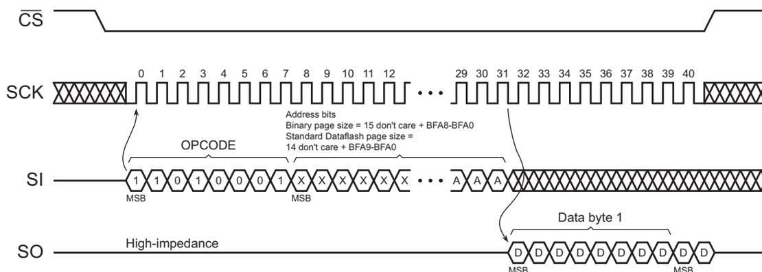
**Figure 22-7. Read Sector Protection Register (Opcode 32H)**
