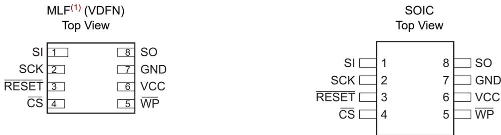
Note: 1. The metal pad on the bottom of the MLF package is floating. This pad can be a "No Connect" or connected to GND.
