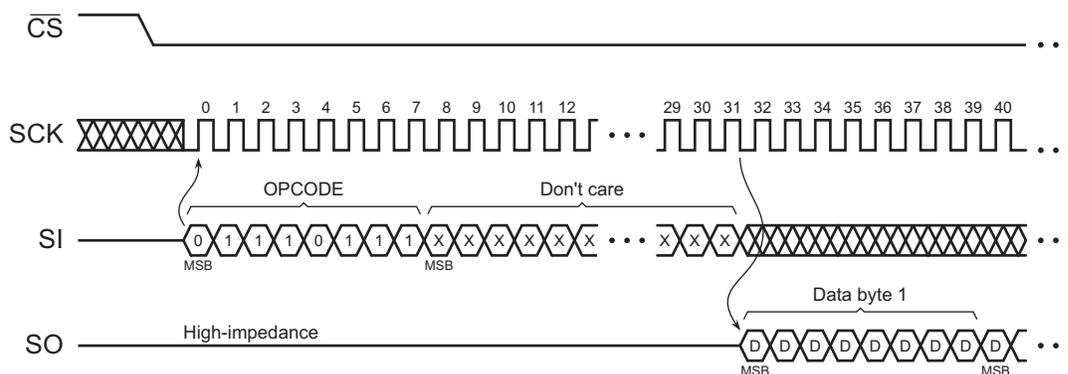
**Figure 22-10. Status Register Read (Opcode D7H)**
