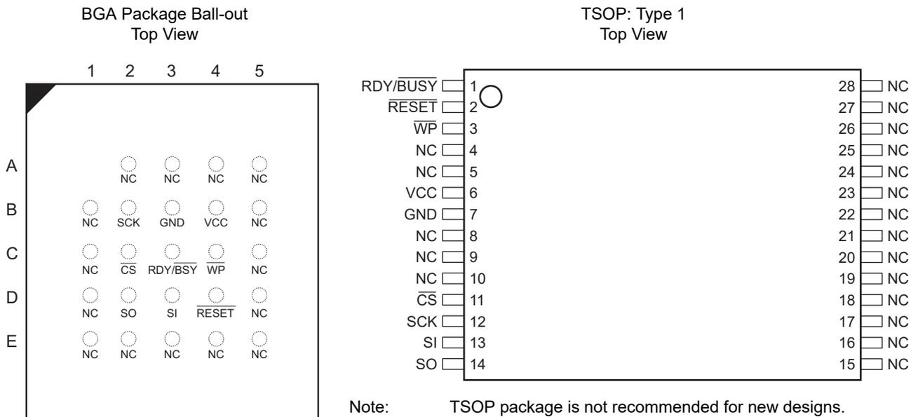
Note: TSOP package is not recommended for new designs. Future die shrinks will support 8-pin packages only.
