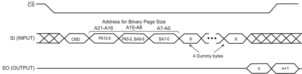
**Figure 21-3. Main Memory Page to Buffer Transfer (Data from Flash Page Read into Buffer)**
