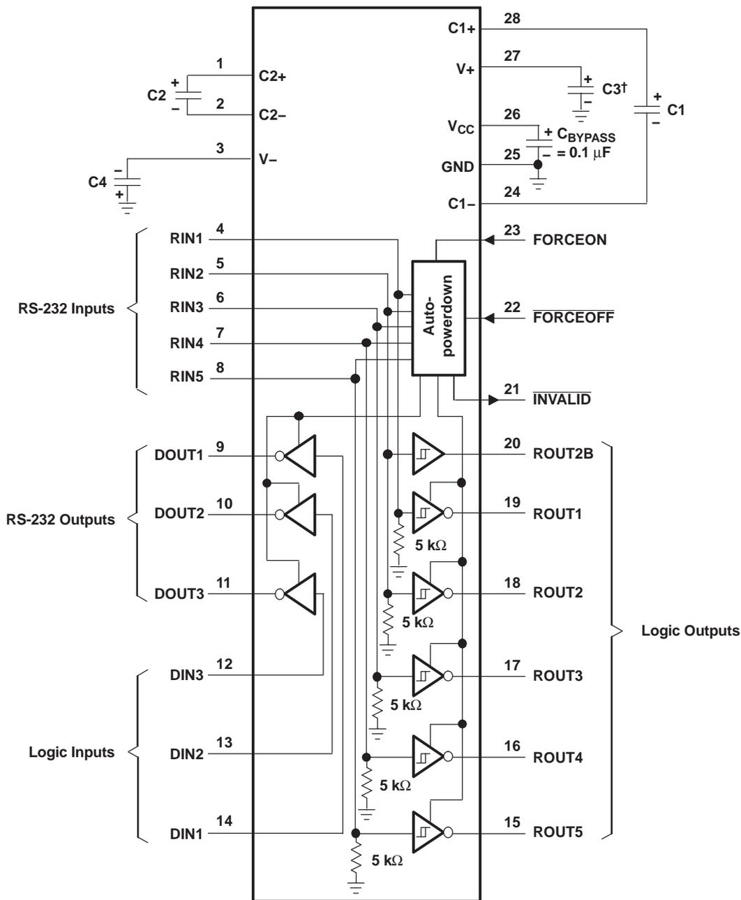
† C3 can be connected to V<sub>CC</sub> or GND.
