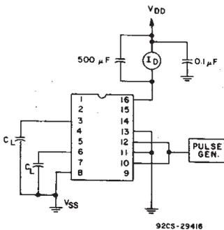
**Fig. 10 – Dynamic power dissipation test circuit.**
