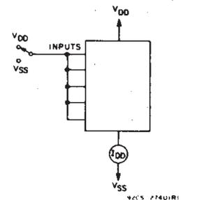
**Fig. 12 – Quiescent device current test circuit.**
