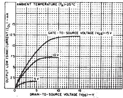
Fig. 3 - Minimum output low (sink) current characteristics.
