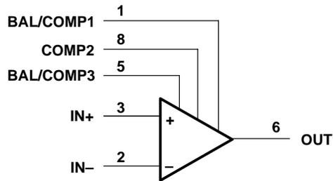
Pin numbers shown are for the D, JG, P, and PS packages.
