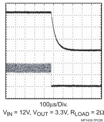
**Load Transient Waveforms**
