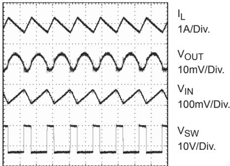
$V_{IN} = 12V$ ,  $V_{OUT} = 3.3V$ ,  $R_{LOAD} = 2\Omega$
