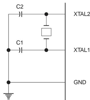
Note: 1. C1, C2 = 30 pF  $\pm$  10 pF for Crystals
