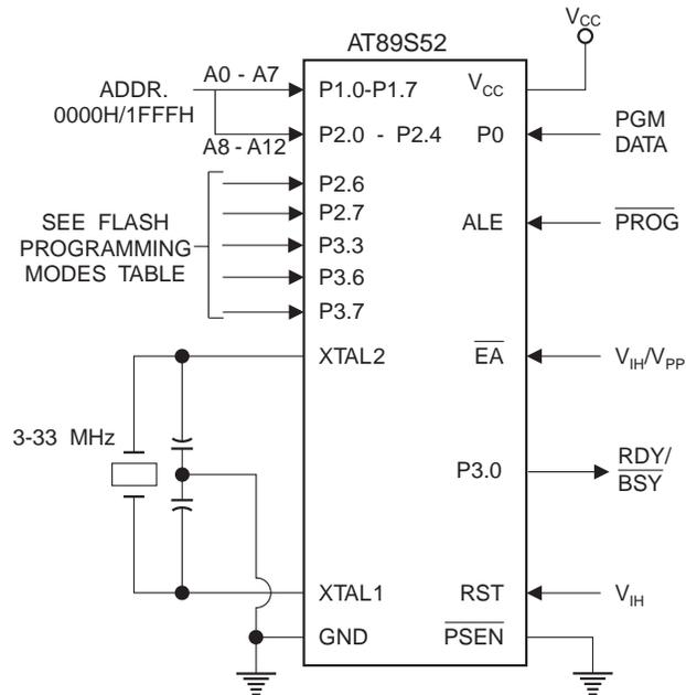
**Figure 10.** Verifying the Flash Memory (Parallel Mode)
