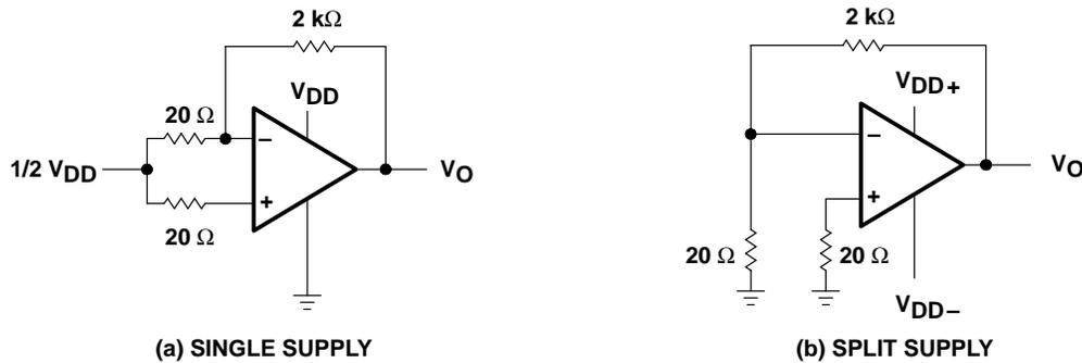
Figure 2. Noise-Test Circuit
