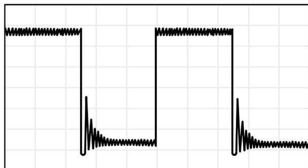
(c)  $C_L = 310 \text{ pF}$ ,  $R_L = \text{NO LOAD}$
