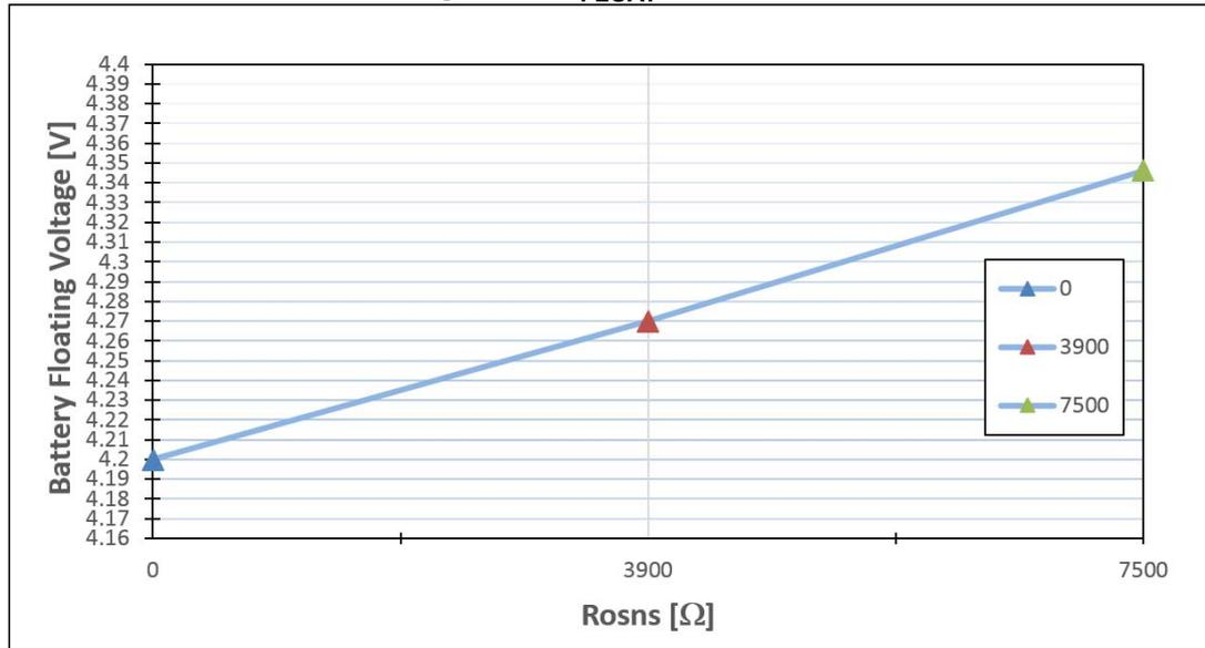
The L6924D works with the selected external components. The test results confirm that their behavior is in line with the design.
