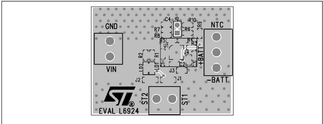
Figure 30. Demonstration board schematic
