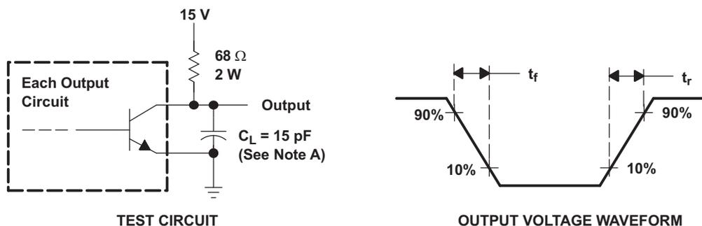
NOTE A:  $C_L$  includes probe and jig capacitance.
