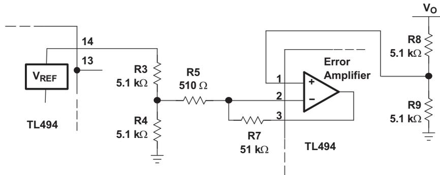
Figure 11. Error-Amplifier Section
