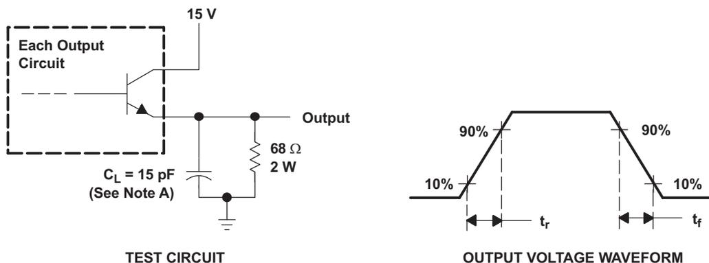
NOTE A:  $C_L$  includes probe and jig capacitance.
