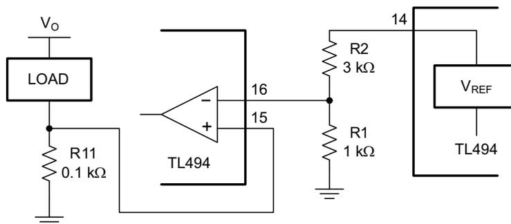
Figure 12. Current-Limiting Circuit
