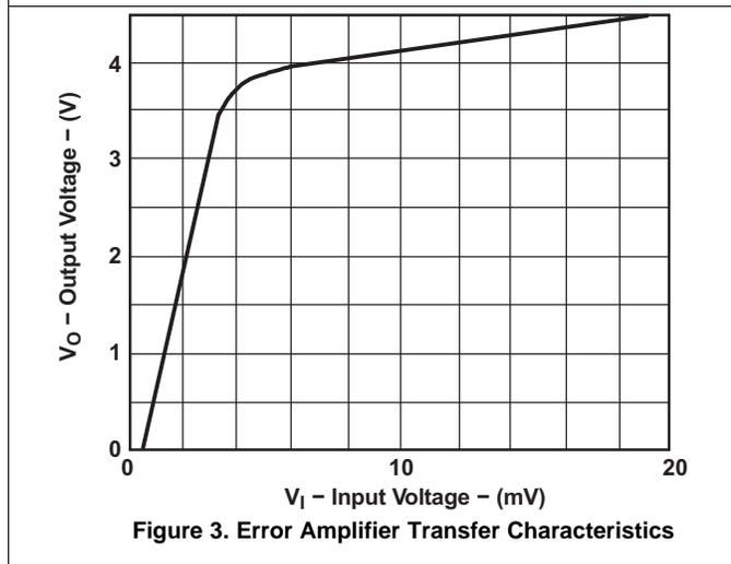
**Figure 3. Error Amplifier Transfer Characteristics**
