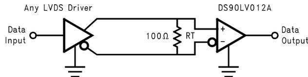
**Figure 7. Point-to-Point Application (DS90LV012A)**
