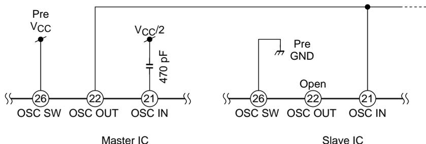
**5. Reduction of Pop Noise Generated when Turning on and Off the Power Supply**
