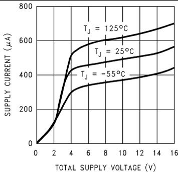
Figure 3. Supply Current vs. Supply Voltage
