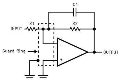
Figure 26. Inverting Amplifier
