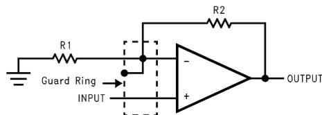
Figure 27. Noninverting Amplifier
