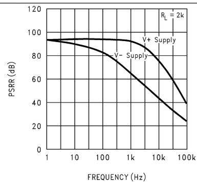
Figure 6. Power Supply Rejection Ratio vs. Frequency
