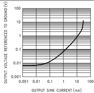
Figure 10. Output Characteristics Sinking Current
