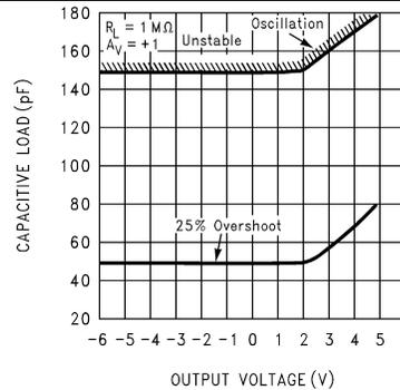
Figure 18. Stability vs. Capacitive Load
