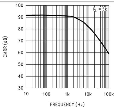
Figure 5. Common-Mode Rejection Ratio vs. Frequency
