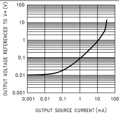
Figure 9. Output Characteristics Sourcing Current
