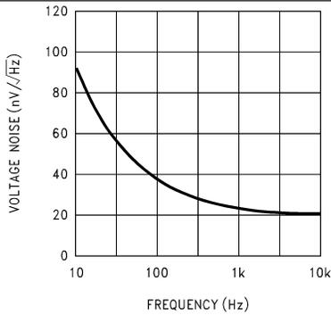
Figure 7. Input Voltage Noise vs. Frequency
