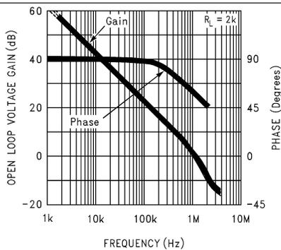
Figure 11. Gain and Phase Response vs. Temperature (-55°C to +125°C)
