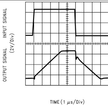
Figure 17. Noninverting Large Signal Pulse Response
