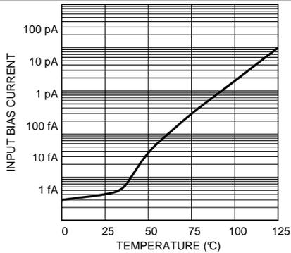
Figure 1. Input Current vs. Temperature
