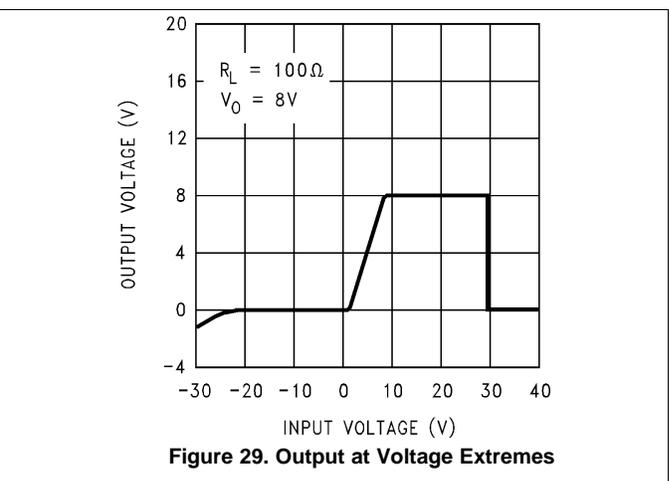
Figure 29. Output at Voltage Extremes
