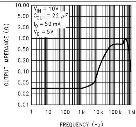
Figure 22. Output Impedance
