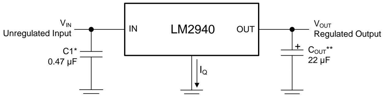
\*Required if regulator is located far from power supply filter.
