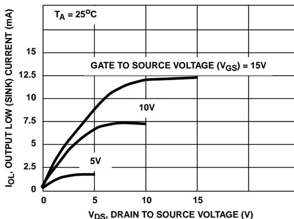
FIGURE 4. MINIMUM OUTPUT LOW (SINK) CURRENT CHARACTERISTICS
