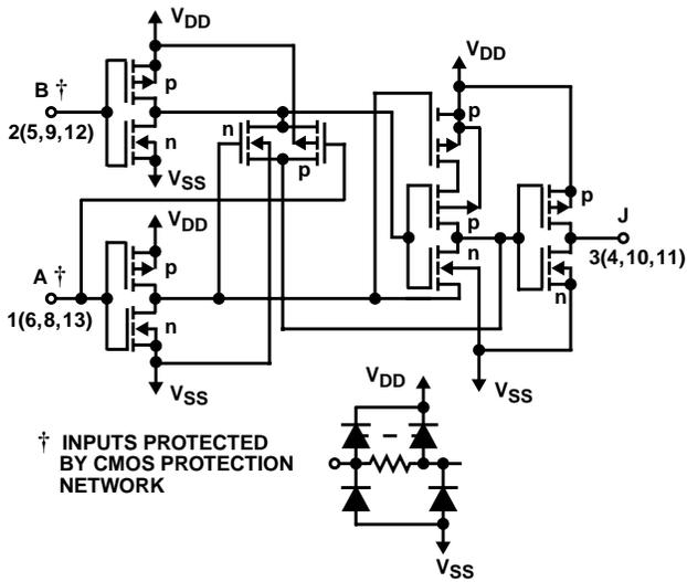
**FIGURE 1. SCHEMATIC DIAGRAM FOR CD4070B
