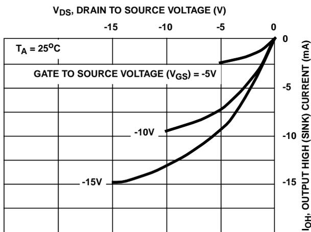
FIGURE 6. MINIMUM OUTPUT HIGH (SOURCE) CURRENT CHARACTERISTICS
