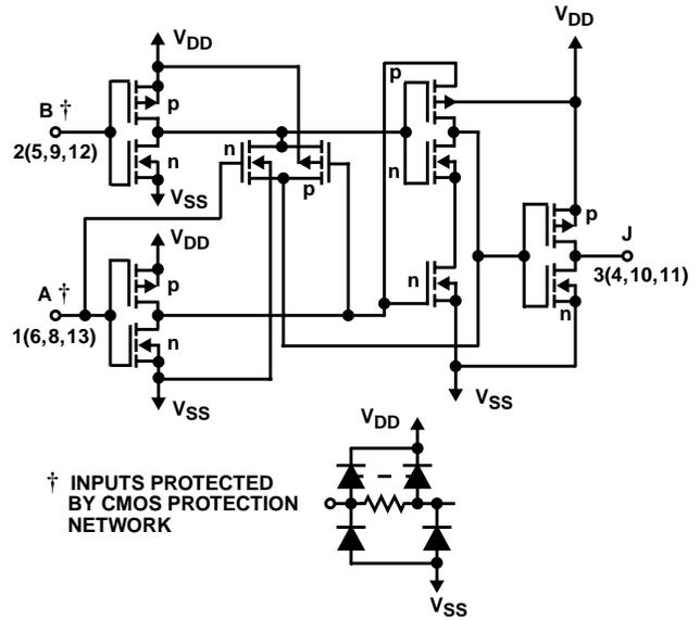
**FIGURE 2. SCHEMATIC DIAGRAM FOR CD4077B
