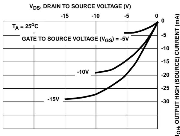
FIGURE 5. TYPICAL OUTPUT HIGH (SOURCE) CURRENT CHARACTERISTICS
