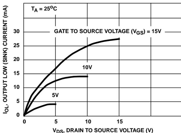
FIGURE 3. TYPICAL OUTPUT LOW (SINK) CURRENT CHARACTERISTICS
