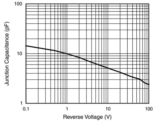
Fig. 5 - Typical Junction Capacitance Per Leg
