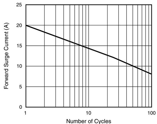
Fig. 2 - Maximum Non-Repetitive Forward Surge Current
