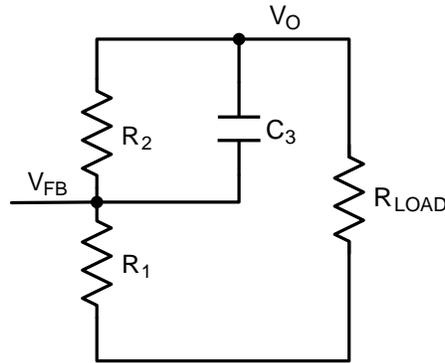
**Figure 20. Setting V<sub>out</sub>**
