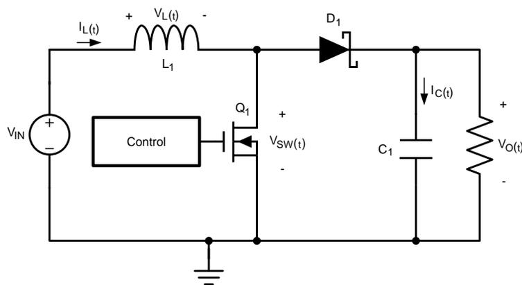
**Figure 13. Simplified Schematic**
