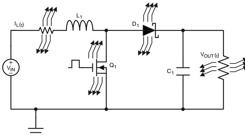
**Figure 47. Thermal Schematic**
