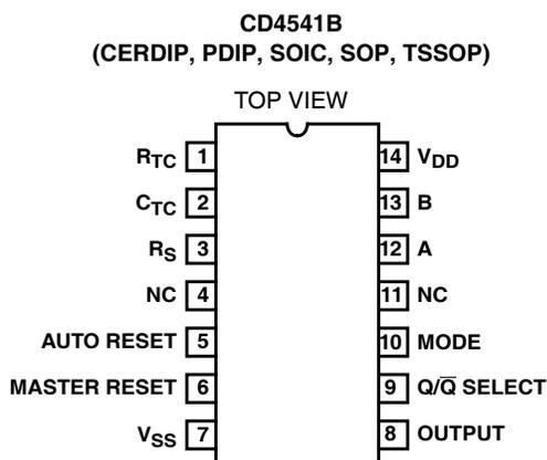
The output from this timer is the Q or  $\bar{Q}$  output from the 8th, 10th, 13th, or 16th counter stage. The desired stage is chosen using time-select inputs A and B (see Frequency Select Table).
