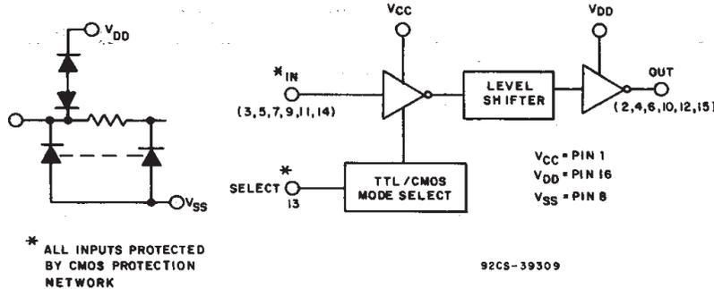
Fig. 1 - Functional diagram for CD4504B.
