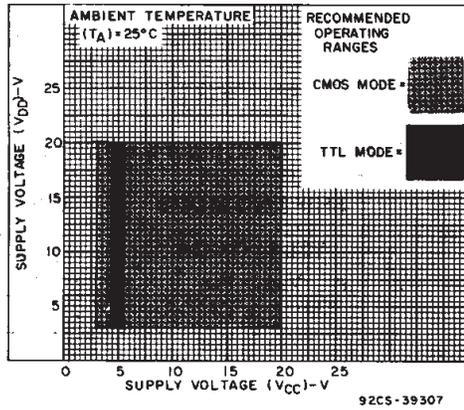
Fig. 11 - High-level supply voltage vs. low-level supply voltage.
