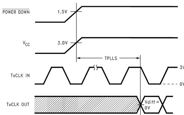
Figure 10. DS90C385A (Transmitter) Phase Lock Loop Set Time
