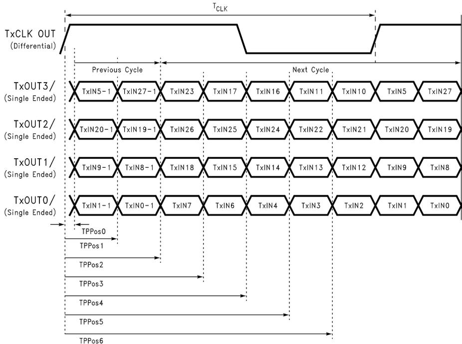
Figure 13. Transmitter LVDS Output Pulse Position Measurement - DS90C385A
