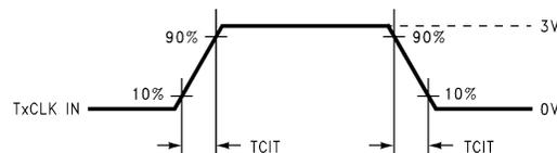
Figure 6. DS90C385A (Transmitter) Input Clock Transition Time
