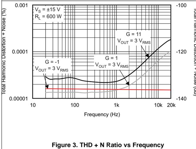
Figure 3. THD + N Ratio vs Frequency
