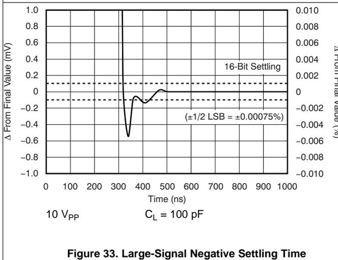
Figure 33. Large-Signal Negative Settling Time
