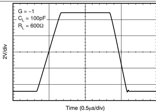
Figure 29. Large-Signal Step Response
