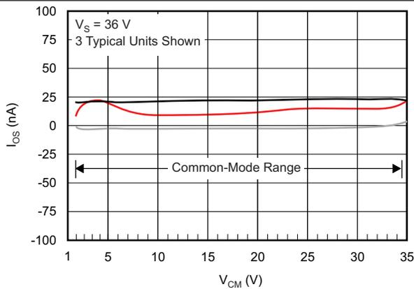
Figure 17. Input Offset Current vs Common-Mode Voltage
