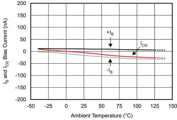
Figure 13.  $I_B$  and  $I_{OS}$  Current vs Temperature
