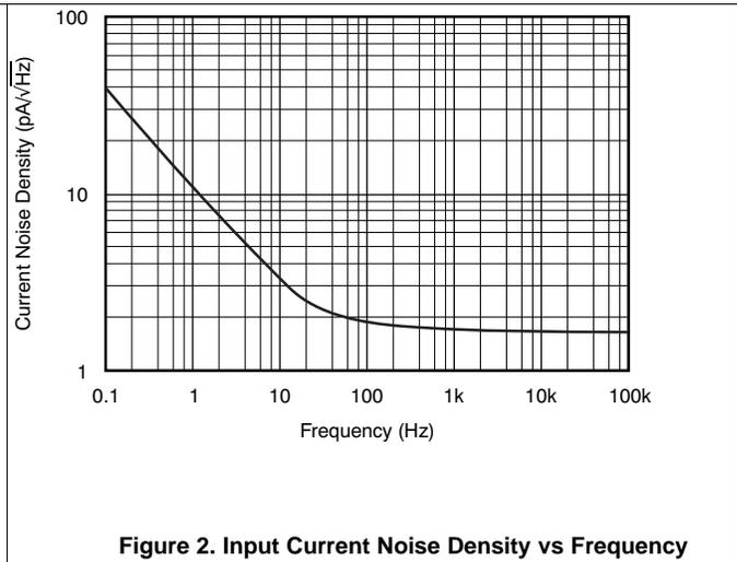
Figure 2. Input Current Noise Density vs Frequency
