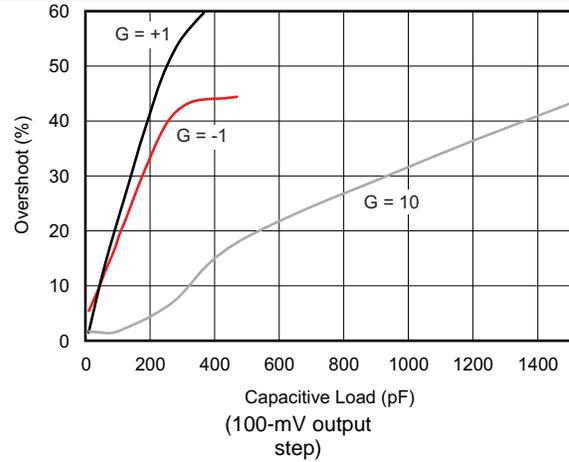
Figure 28. Small-Signal Overshoot vs Capacitive Load
