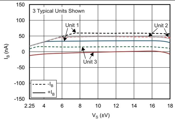
Figure 18. Input Bias Current vs Supply Voltage
