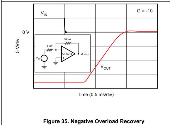
Figure 35. Negative Overload Recovery
