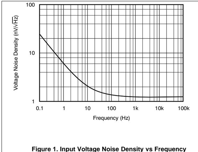
Figure 1. Input Voltage Noise Density vs Frequency
