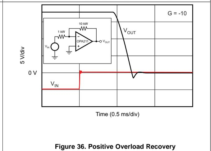
Figure 36. Positive Overload Recovery
