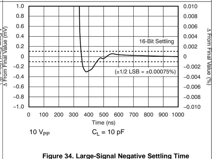
Figure 34. Large-Signal Negative Settling Time
