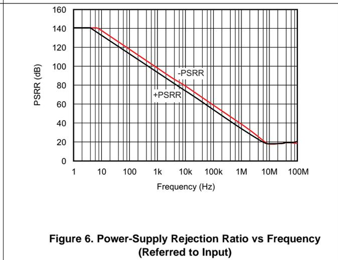
Figure 6. Power-Supply Rejection Ratio vs Frequency (Referred to Input)
