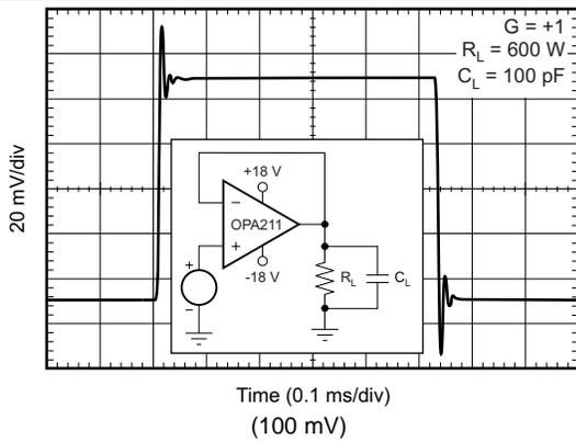
Figure 27. Small-Signal Step Response
