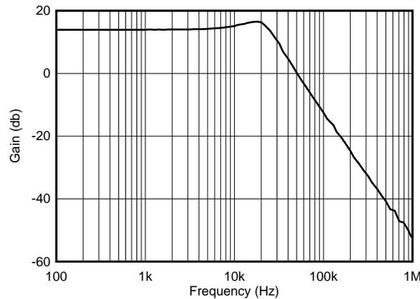
**Figure 50. OPAx211 2nd-Order 25-kHz, Chebyshev, Low-Pass Filter**
