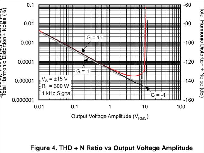
Figure 4. THD + N Ratio vs Output Voltage Amplitude
