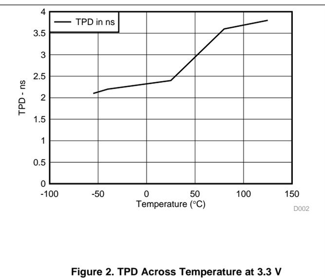
Figure 2. TPD Across Temperature at 3.3V
