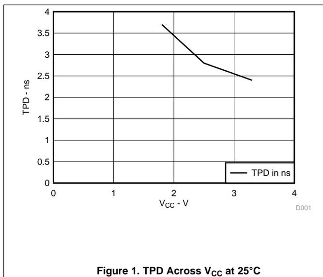
Figure 1. TPD Across V<sub>CC</sub> at 25°C
