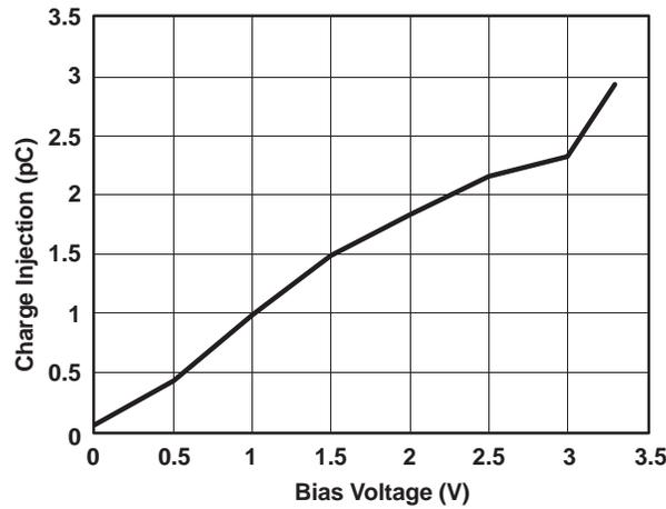
Figure 5. Charge Injection ( $Q_C$ ) vs Bias Voltage
