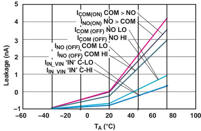
Figure 4. Leakage Current vs Temperature ( $V_+ = 5.5\text{ V}$ )
