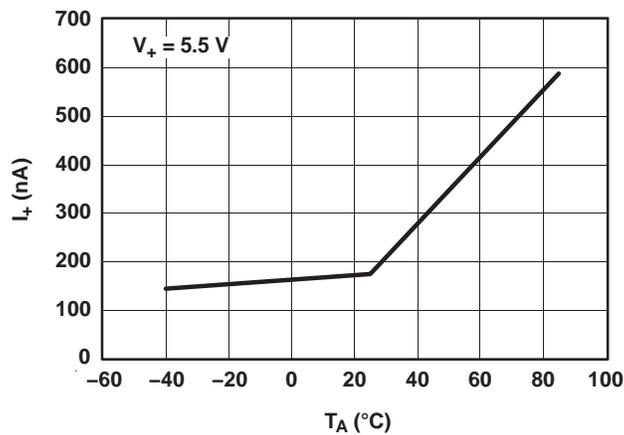
Figure 12. Power-Supply Current vs Temperature ( $V_+ = 5\text{ V}$ )
