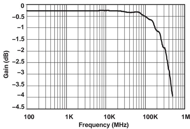
Figure 9. Bandwidth ( $V_+ = 5$  V)
