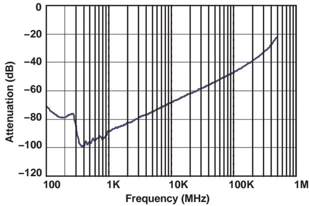
Figure 10. OFF Isolation ( $V_+ = 5\text{ V}$ )
