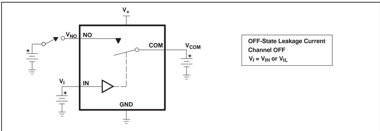
Figure 14. OFF-State Leakage Current ( $I_{COM(OFF)}$ ,  $I_{NO(OFF)}$ )
