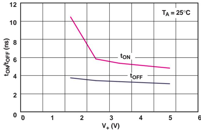
Figure 6.  $t_{ON}$  and  $t_{OFF}$  vs Supply Voltage
