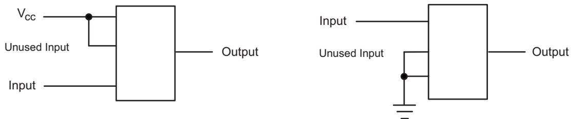
Figure 7. Layout Diagram
