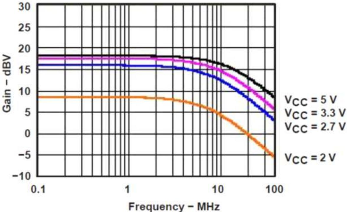
**Figure 6. Open-Loop Gain**
