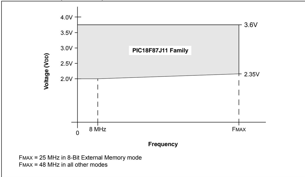
FIGURE 28-2: PIC18F87J11 FAMILY VOLTAGE-FREQUENCY GRAPH, REGULATOR DISABLED (INDUSTRIAL)<sup>0</sup>
