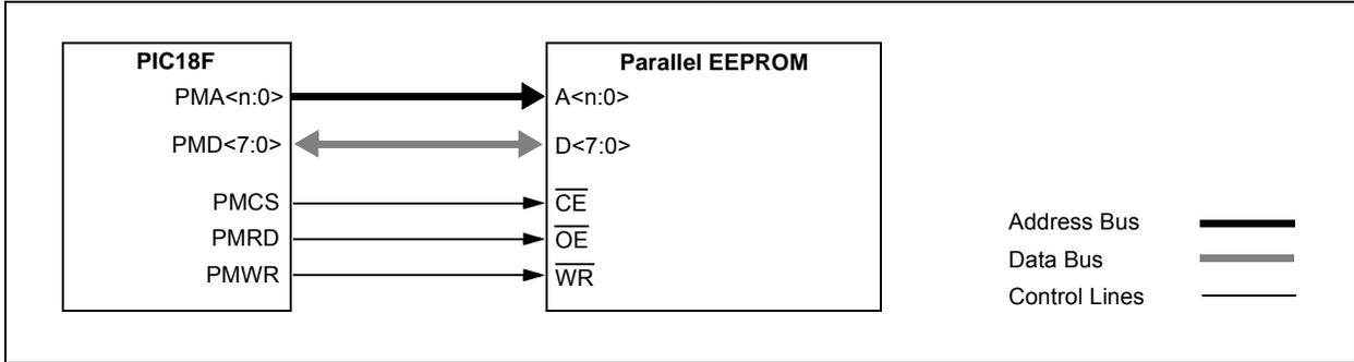
**FIGURE 12-31: PARALLEL EEPROM EXAMPLE (UP TO 15-BIT ADDRESS, 16-BIT DATA)**
