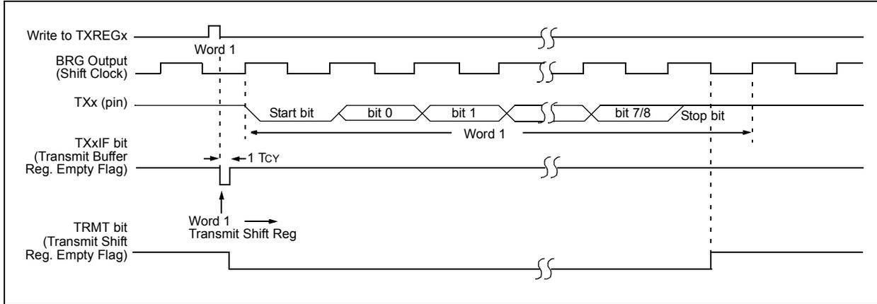
**FIGURE 21-5: ASYNCHRONOUS TRANSMISSION (BACK-TO-BACK)**
