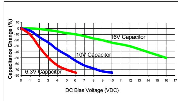
When selecting a ceramic capacitor to be used with the VDDCORE voltage regulator, it is suggested to select a high-voltage rating, so that the operating voltage is a small percentage of the maximum rated capacitor voltage. For example, choose a ceramic capacitor rated at 16V for the 2.5V VDDCORE voltage. Suggested capacitors are shown in [Table 2-1](#).
