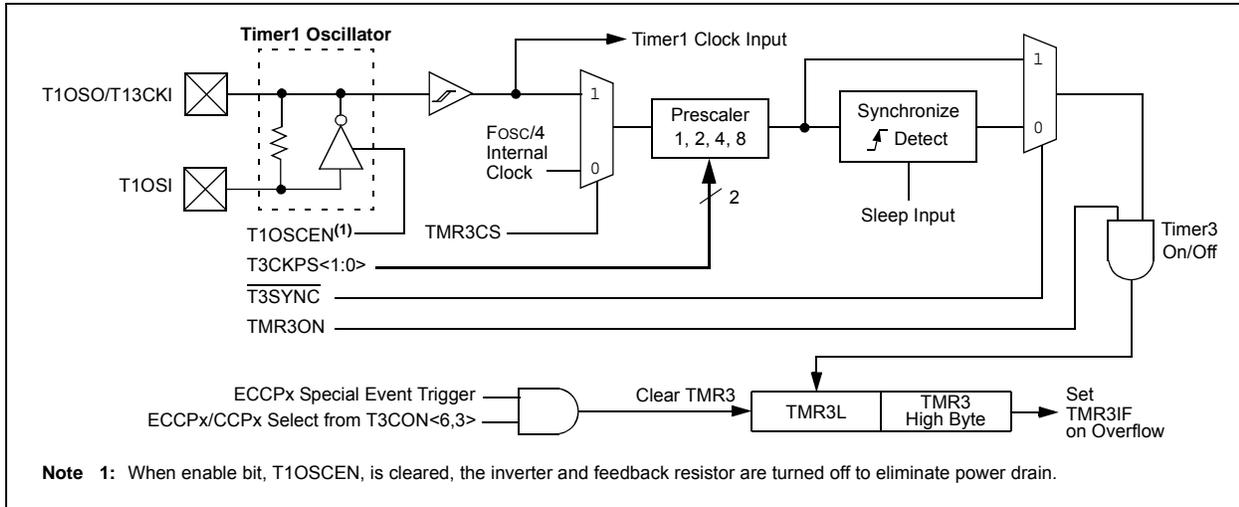
**FIGURE 16-2: TIMER3 BLOCK DIAGRAM (16-BIT READ/WRITE MODE)**
