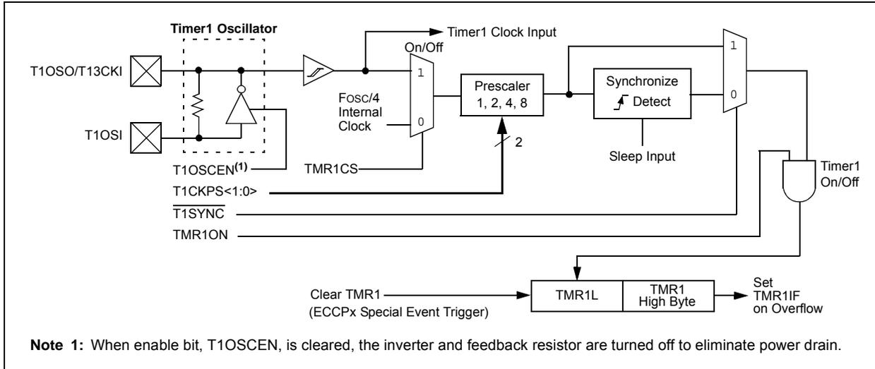
**FIGURE 14-2: TIMER1 BLOCK DIAGRAM (16-BIT READ/WRITE MODE)**
