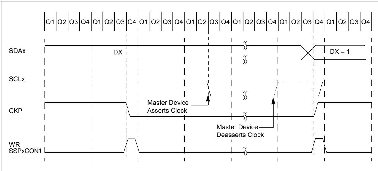
**FIGURE 20-15: I<sup>2</sup>C™ SLAVE MODE TIMING WITH SEN = 1 (RECEPTION, 7-BIT ADDRESS)**
