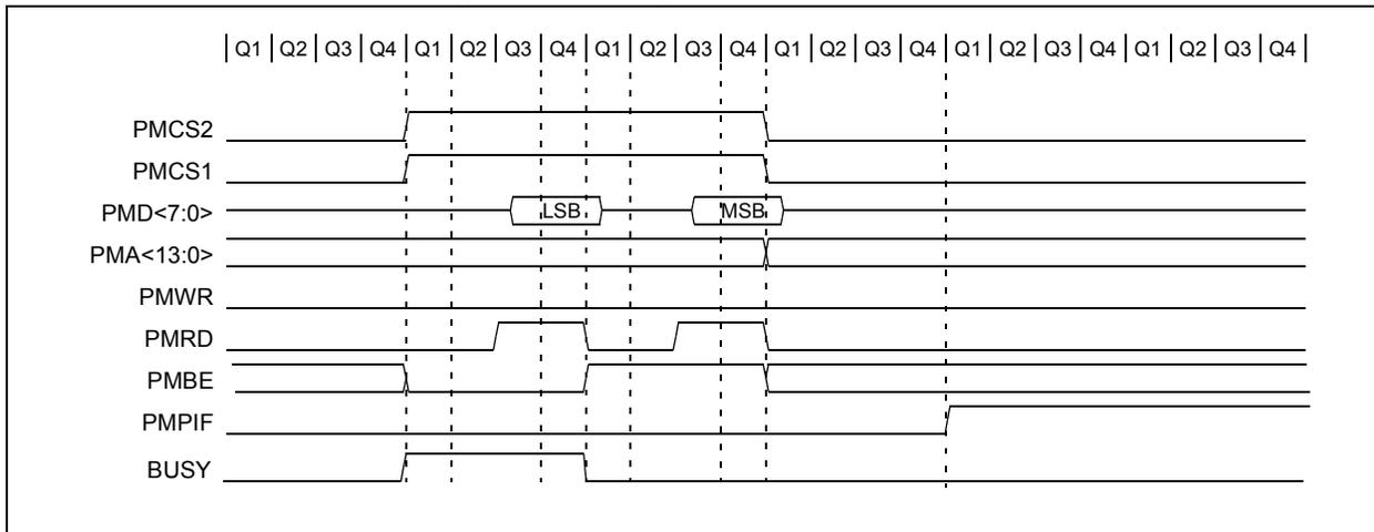
**FIGURE 12-22: WRITE TIMING, 16-BIT DATA, DEMULTIPLEXED ADDRESS**
