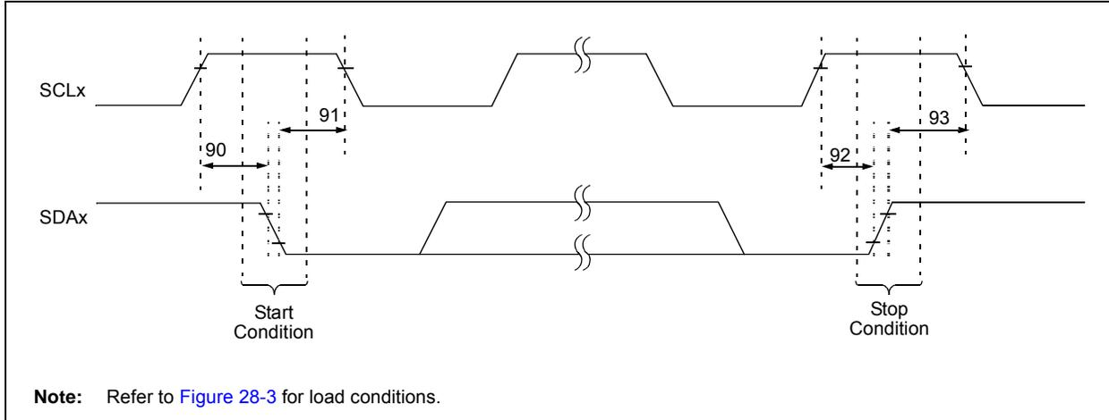
**TABLE 28-24: I<sup>2</sup>C™ BUS START/STOP BITS REQUIREMENTS (SLAVE MODE)**
