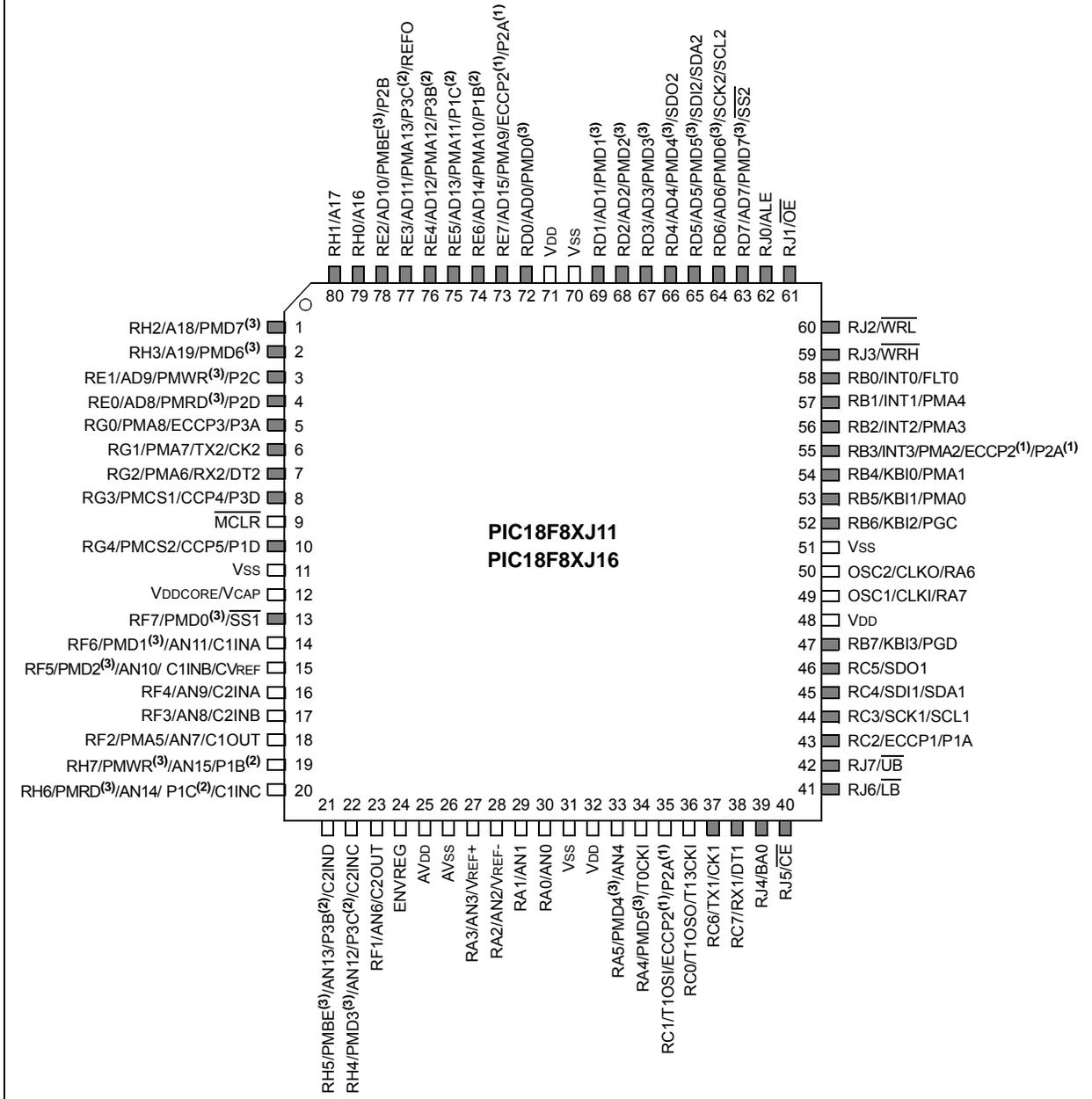
**Legend:** Shaded pins indicate pins that are tolerant up to +5.5V.
