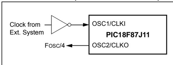
An external clock source may also be connected to the OSC1 pin in the HS mode, as shown in [Figure 3-4](#). In this configuration, the divide-by-4 output on OSC2 is not available. Current consumption in this configuration will be somewhat higher than EC mode, as the internal oscillator's feedback circuitry will be enabled (in EC mode, the feedback circuit is disabled).
