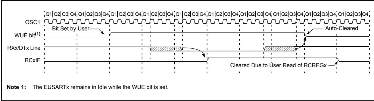
**FIGURE 21-9: AUTO-WAKE-UP BIT (WUE) TIMINGS DURING SLEEP**
