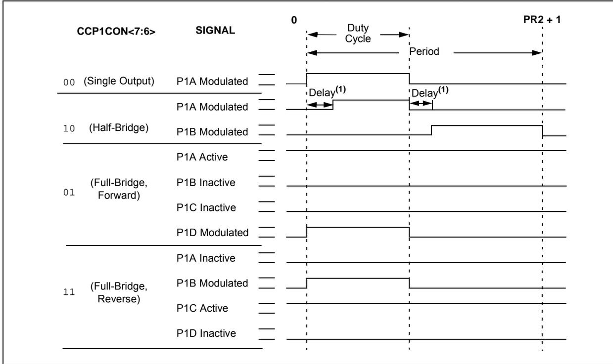
**FIGURE 19-3: PWM OUTPUT RELATIONSHIPS (ACTIVE-LOW STATE)**
