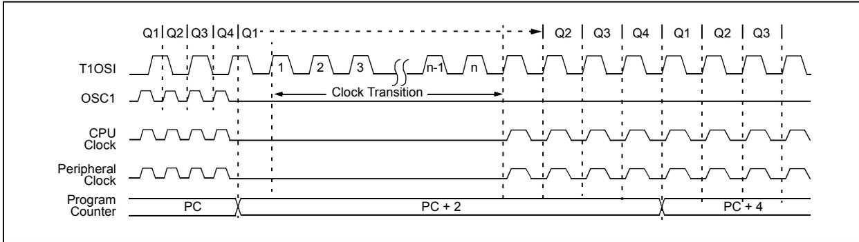
**FIGURE 4-2: TRANSITION TIMING FROM SEC\_RUN MODE TO PRI\_RUN MODE (HSPDLL)**
