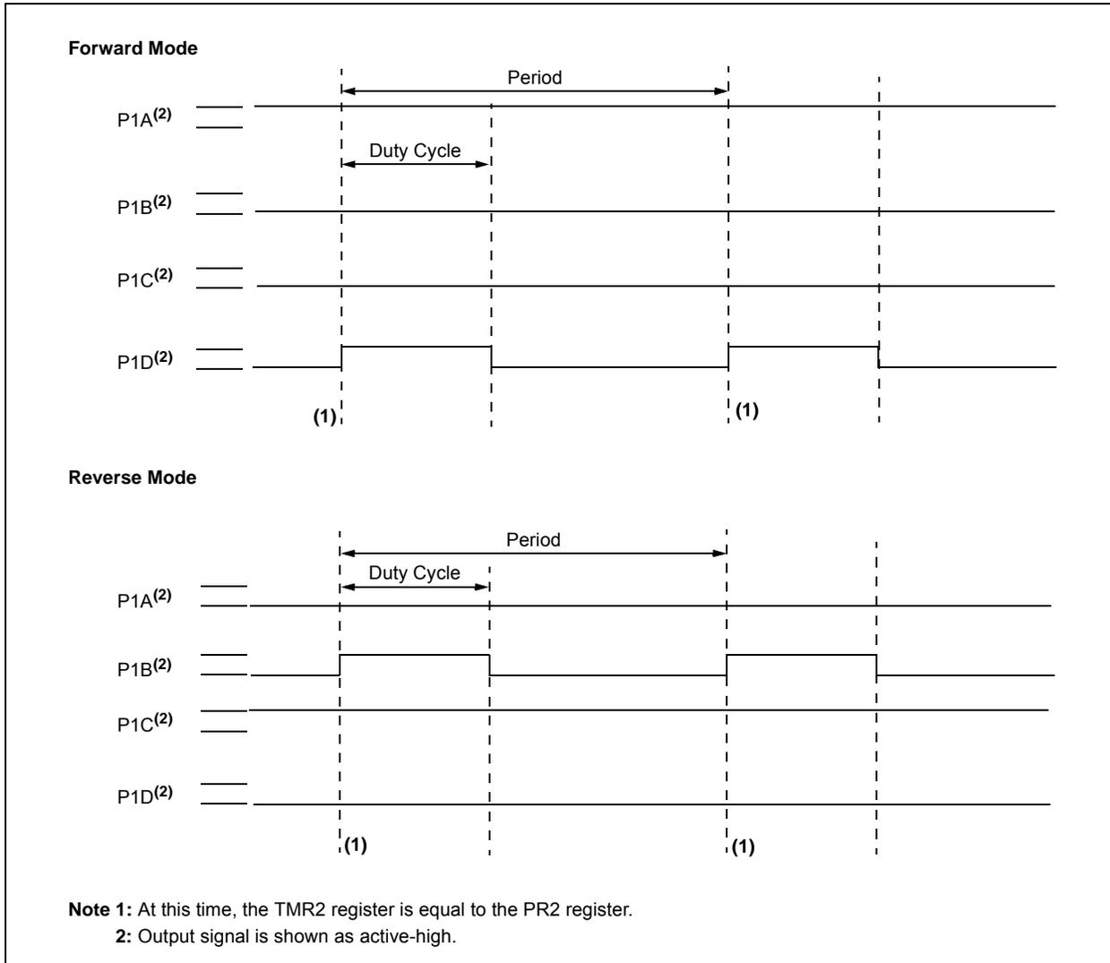
**FIGURE 19-7: EXAMPLE OF FULL-BRIDGE OUTPUT APPLICATION**
