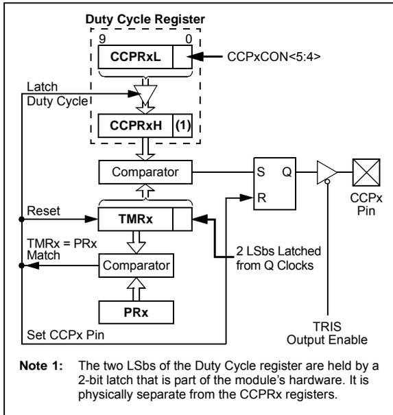
A PWM output (Figure 18-5) has a time base (period) and a time that the output stays high (duty cycle). The frequency of the PWM is the inverse of the period (1/period).
