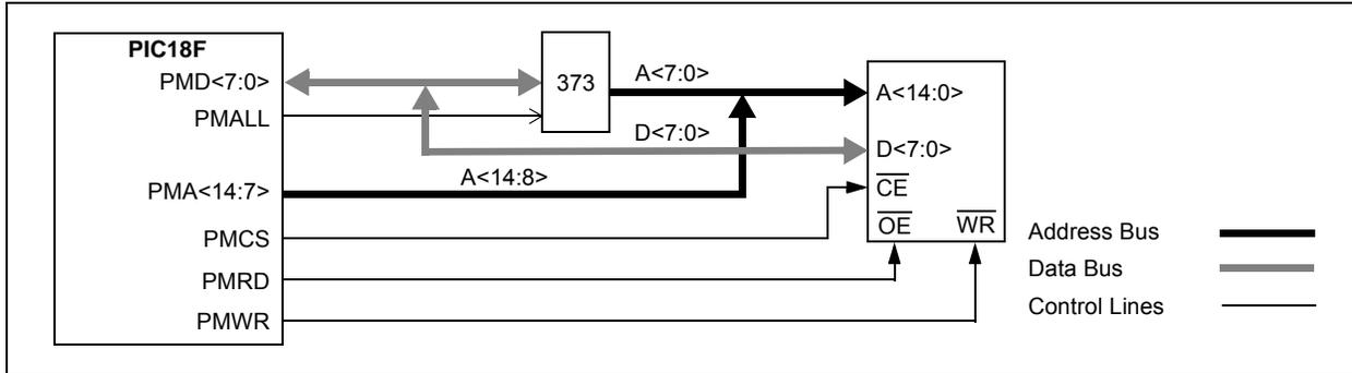
**FIGURE 12-29: EXAMPLE OF AN 8-BIT MULTIPLEXED ADDRESS AND DATA APPLICATION**
