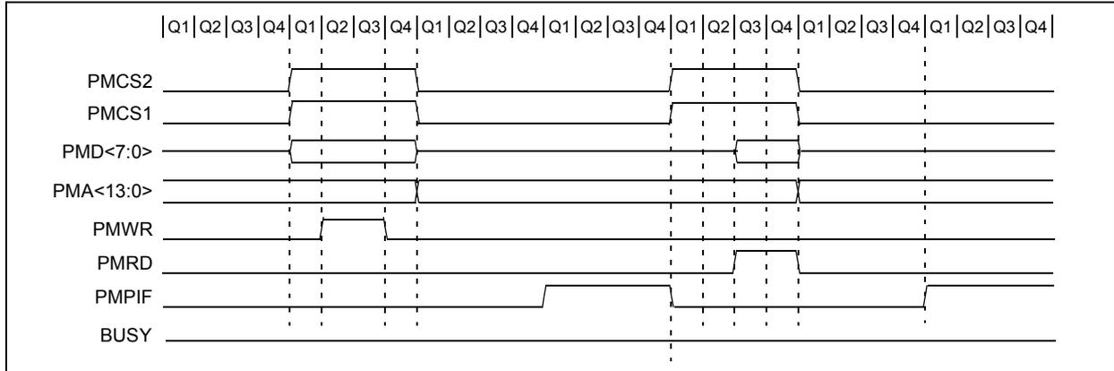
**FIGURE 12-13: READ TIMING, 8-BIT DATA, PARTIALLY MULTIPLEXED ADDRESS**
