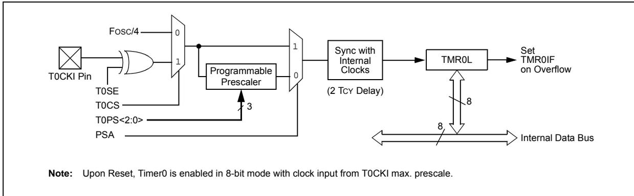
**FIGURE 13-2: TIMER0 BLOCK DIAGRAM (16-BIT MODE)**
