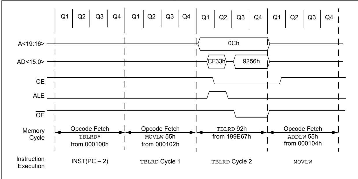
**FIGURE 8-5: EXTERNAL MEMORY BUS TIMING FOR SLEEP (EXTENDED MICROCONTROLLER MODE)**
