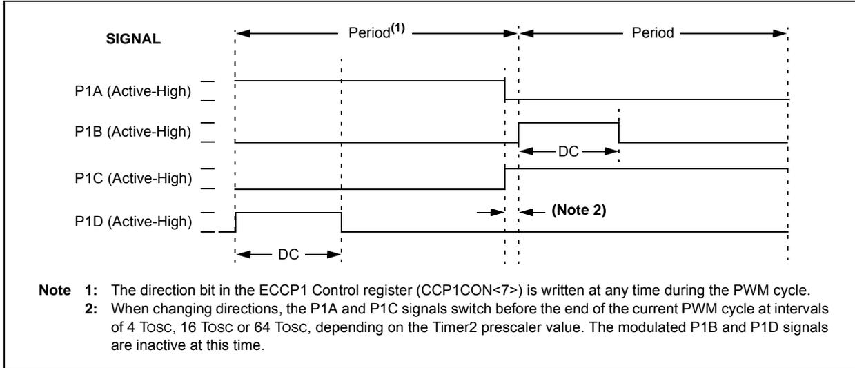
**FIGURE 19-9: PWM DIRECTION CHANGE AT NEAR 100% DUTY CYCLE**
