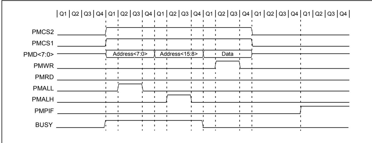
**FIGURE 12-21: READ TIMING, 16-BIT DATA, DEMULTIPLEXED ADDRESS**
