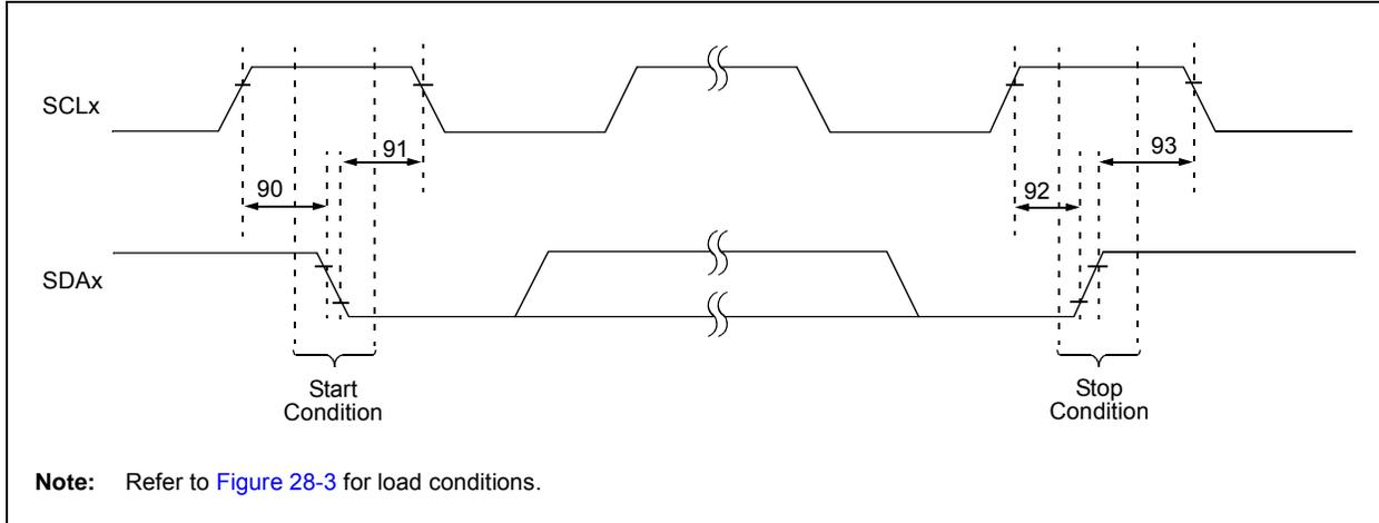
**TABLE 28-26: MSSPx I<sup>2</sup>C™ BUS START/STOP BITS REQUIREMENTS**
