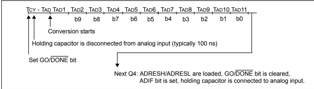
**FIGURE 22-4: A/D CONVERSION TAD CYCLES ( $\text{ACQT}\langle 2:0 \rangle = 010, \text{TACQ} = 4 \text{ TAD}$ )**
