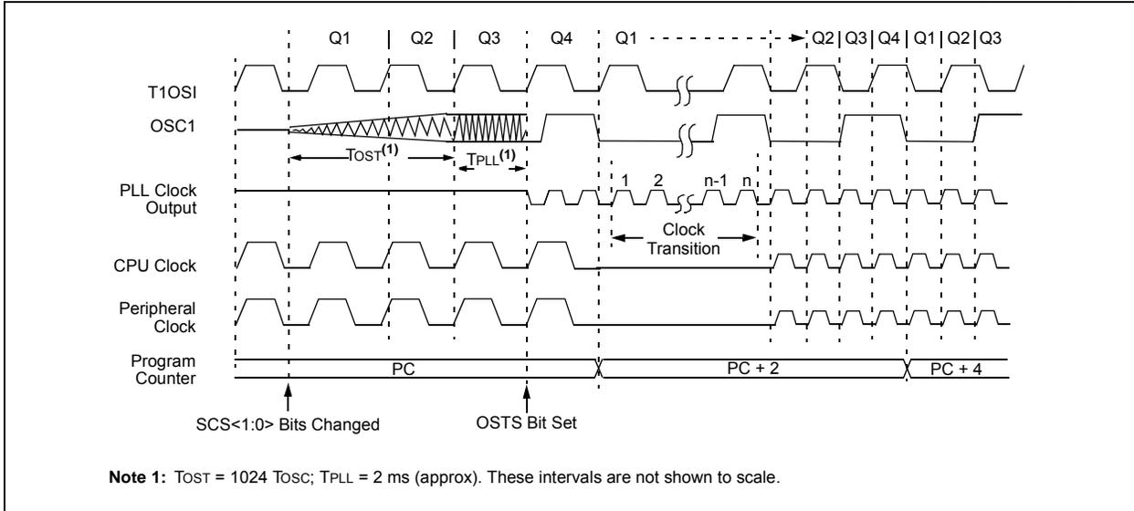
**Note 1:**  $T_{OST} = 1024 T_{OSC}$ ;  $T_{PLL} = 2 \text{ ms (approx)}$ . These intervals are not shown to scale.
