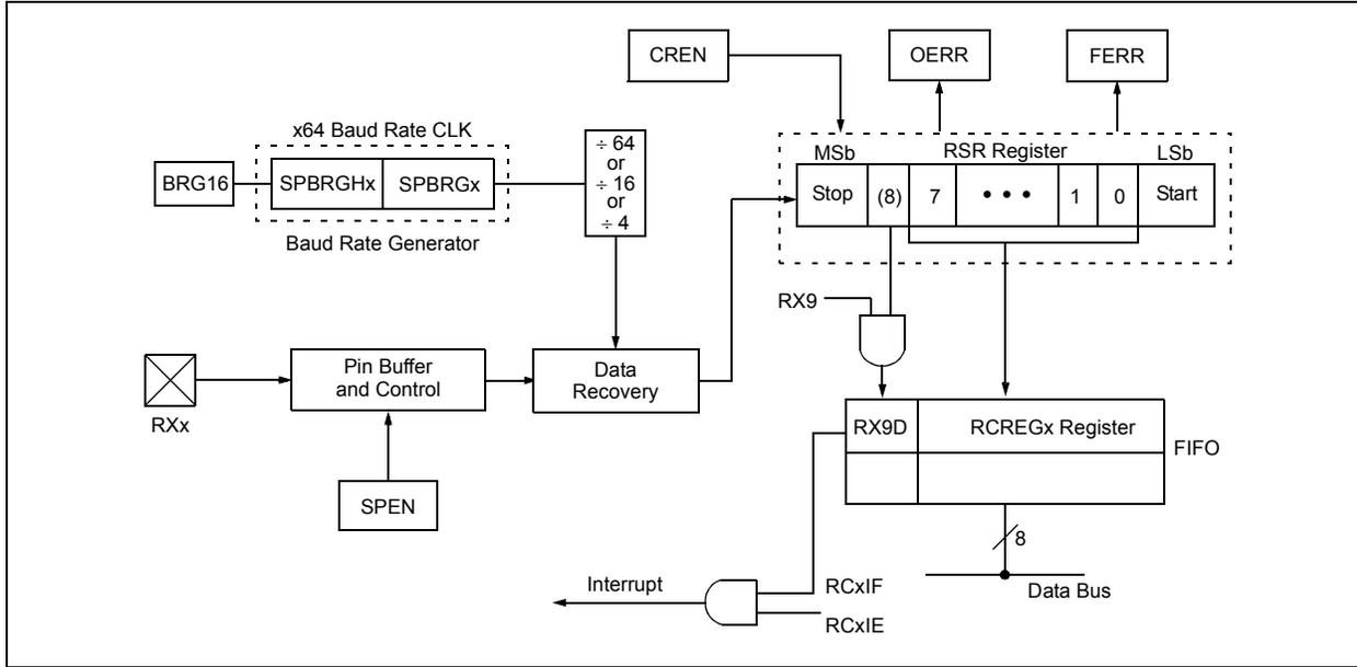
**FIGURE 21-7: ASYNCHRONOUS RECEPTION**
