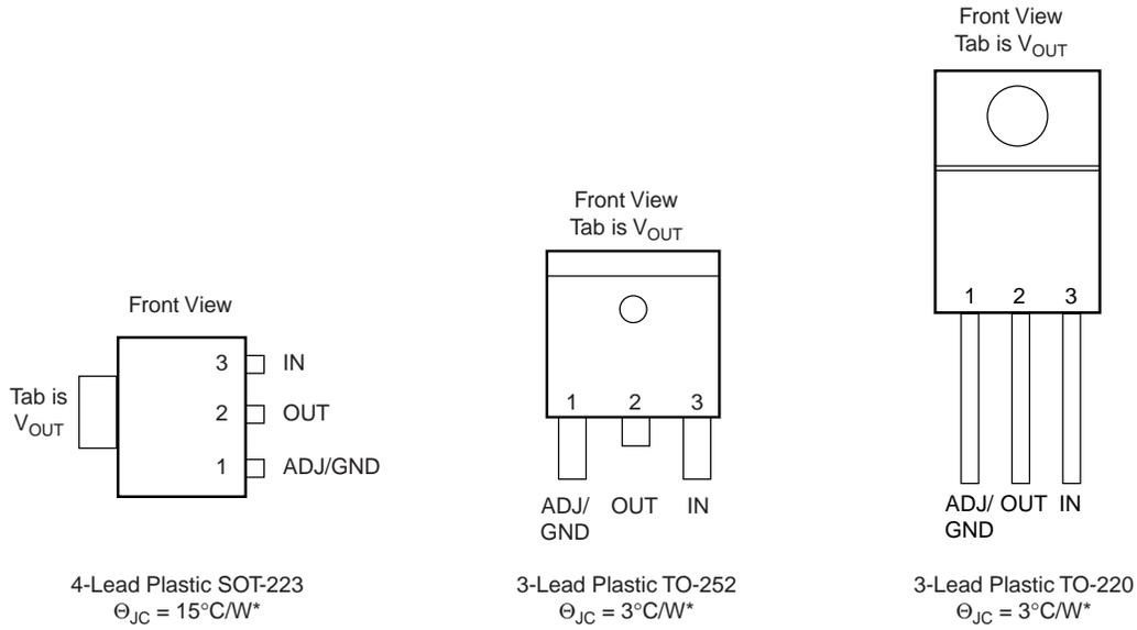
\*With package soldered to 0.5 square inch copper area over backside ground plane or internal power plane,  $\theta_{JA}$  can vary from 30°C/W to more than 50°C/W. Other mounting techniques may provide better thermal resistance than 30°C/W.
