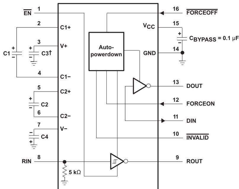
† C3 can be connected to  $V_{CC}$  or GND.
