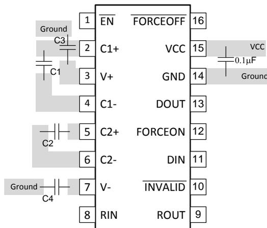
**Figure 10. Layout Diagram**
