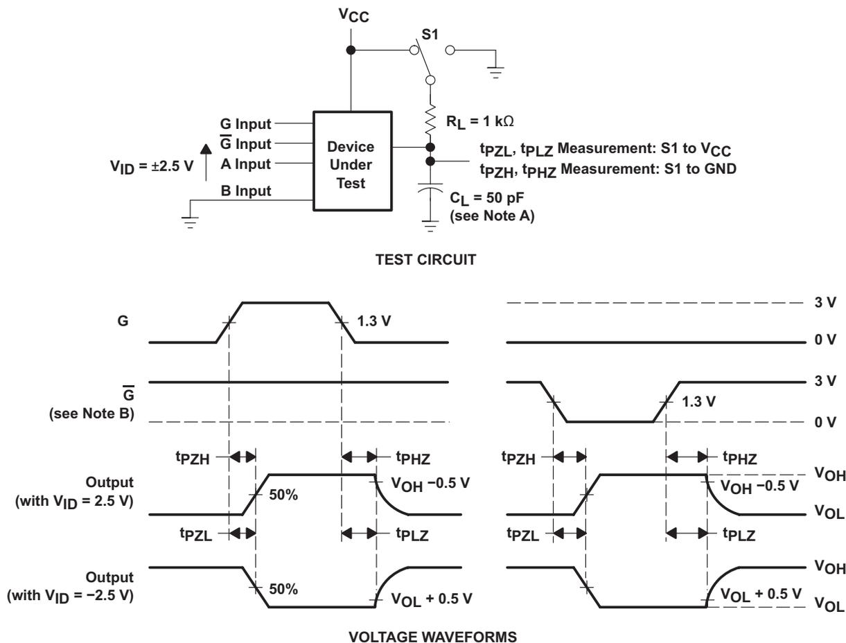
A.  $C_L$  includes probe and jig capacitance.
