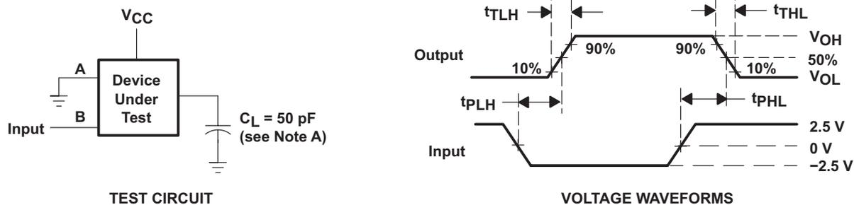
A.  $C_L$  includes probe and jig capacitance.
