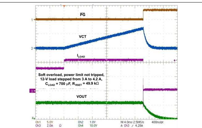
Figure 18. 12-V Soft Overload, 3 A to 4.2 A, Power Limit Not Tripped
