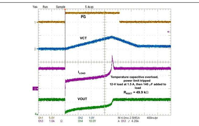
Figure 16. 12 V, 140 μF Added to 8-Ω Load
