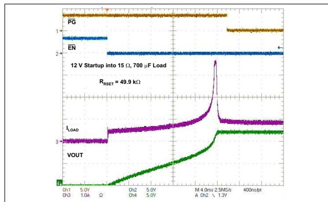
Figure 15. 12-V Startup into 15-Ω, 700-μF Load
