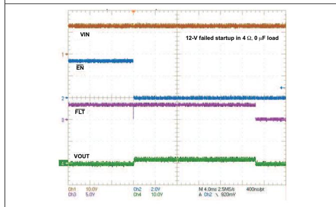
Figure 17. 12-V Failed Startup into 4-Ω Load
