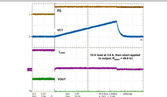
Figure 20. 12-V Hard Overload, 3.6-A Load then Short
