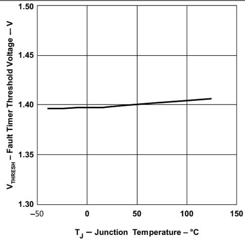
Figure 2. Fault Timer Threshold Voltage vs Junction Temperature
