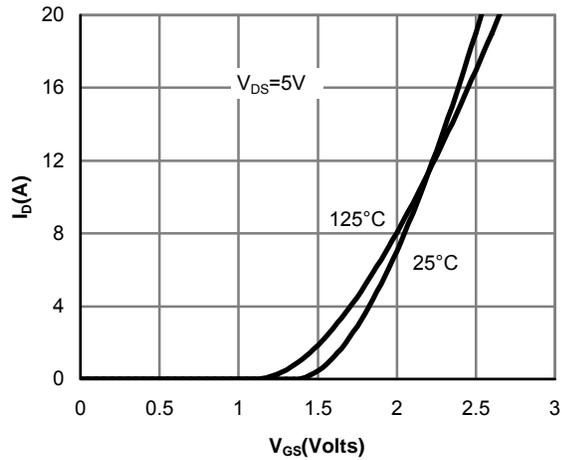
Figure 2: Transfer Characteristics
