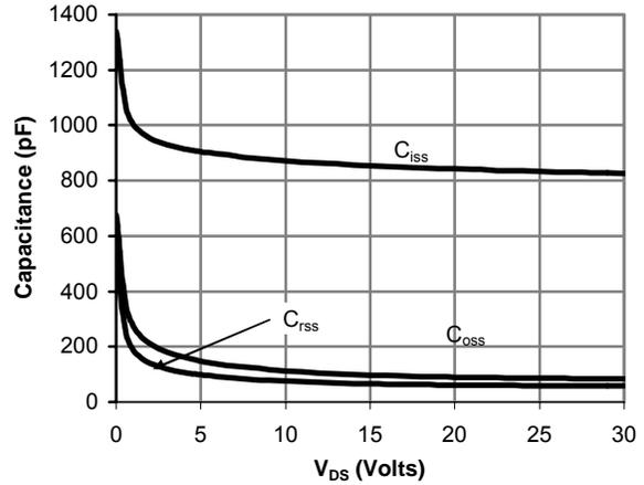
Figure 8: Capacitance Characteristics
