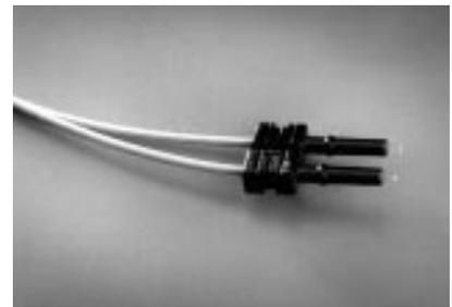
Manually press connectors together in the center of the arrangement. Then latch by pressing on the sides of each connector. As with the simplex version, connectors are secured when top halves latch into the ferrule halves.
