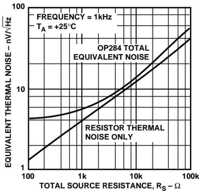
Figure 46. OP284 Total Noise vs. Source Resistance
