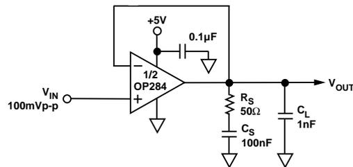
Figure 53. Snubber Network Compensates for Capacitive Load
