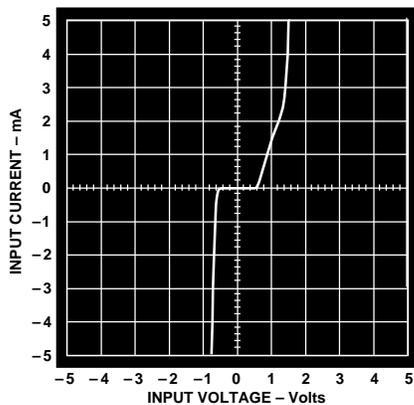
Figure 43. Input Overvoltage I-V Characteristics of the OP284
