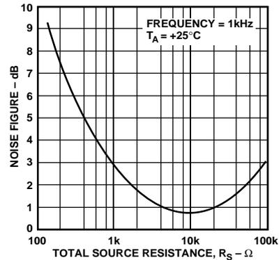
Figure 47. OP284 Noise Figure vs. Source Resistance
