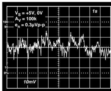
Figure 34. 0.1 Hz to 10 Hz Noise
