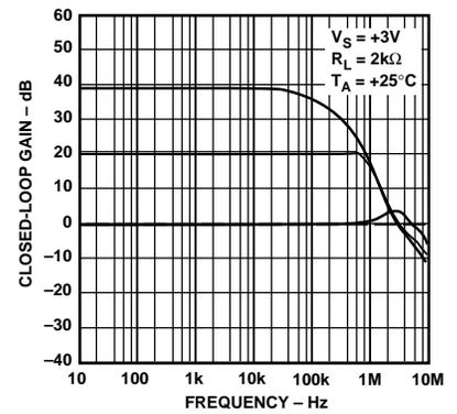
Figure 19. Closed-Loop Gain vs. Frequency (2 kΩ Load)
