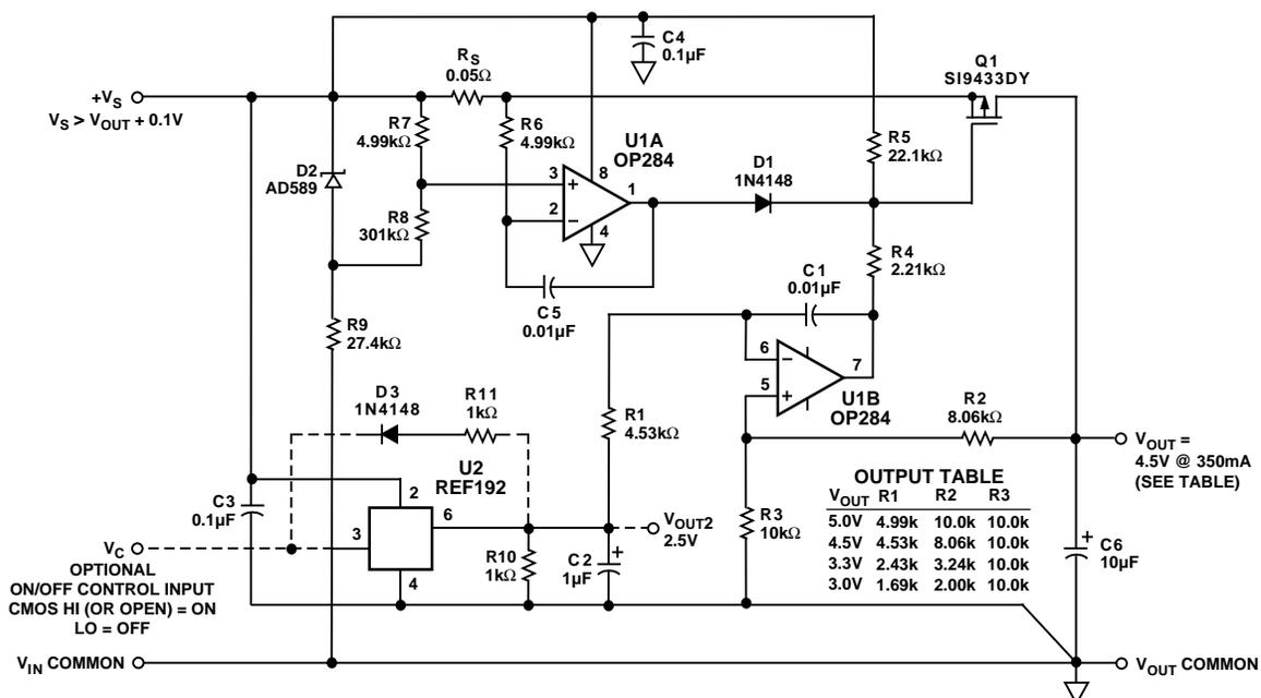
Figure 55. A Low Dropout Regulator with Current Limiting
