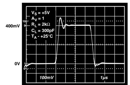
Figure 37. Small Signal Transient Response
