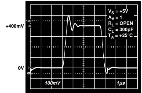
Figure 36. Small Signal Transient Response
