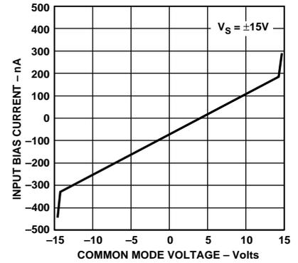
Figure 8. Input Bias Current vs. Common-Mode Voltage
