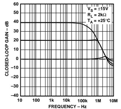
Figure 18. Closed-Loop Gain vs. Frequency (2 kΩ Load)
