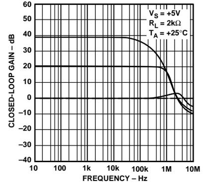
Figure 17. Closed-Loop Gain vs. Frequency (2 kΩ Load)
