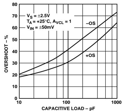
Figure 27. Small Signal Overshoot vs. Capacitive Load
