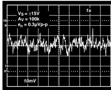
Figure 33. 0.1 Hz to 10 Hz Noise
