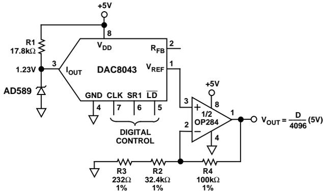
Figure 51. A +5 V Only, 12-Bit DAC Swings Rail-to-Rail
