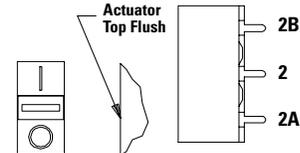
Note: Orientation of actuator markings and terminals.
