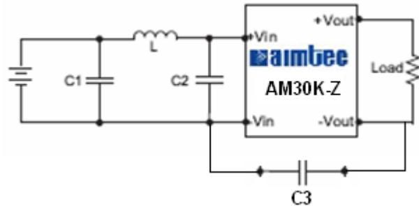
**Note A:** An external filter capacitor is required if the module has to meet EN61000-4-4 and EN61000-4-5. The filter capacitor Aimtec suggests: 1000uF, 100V.
