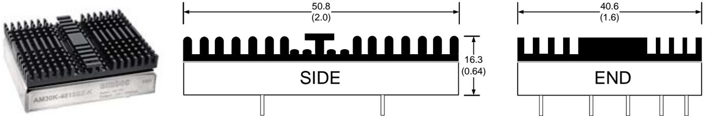
Notes: Add "-K" suffix for ordering, heat sink is affixed with thermally dissipative adhesive tape. See derating graph for temperature performance. Heat sink material is anodized (black) aluminum, adds weight 17g to total mass (65g). Thermal impedance of converter is: with heatsink 8.7 °C/W and 10°C/W without heat sink.
