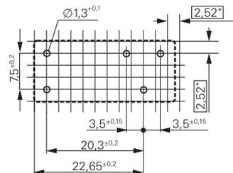
\*) With the recommended PCB hole sizes a grid pattern from 2.5mm to 2.54mm can be used.
