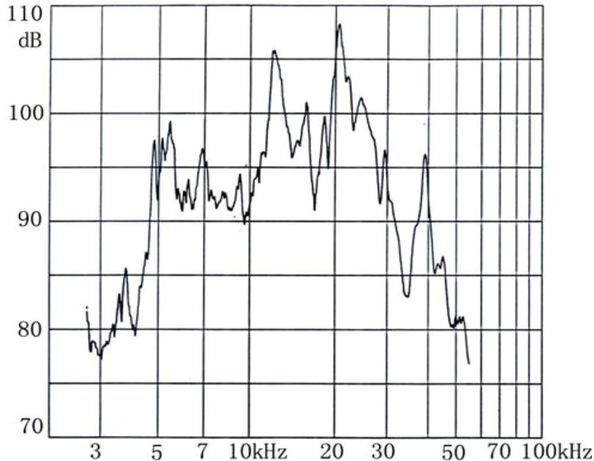
**Note:** Input Voltage 2.83Vrms sine wave
