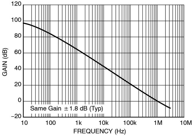
Figure 1. Open Loop Frequency Response
