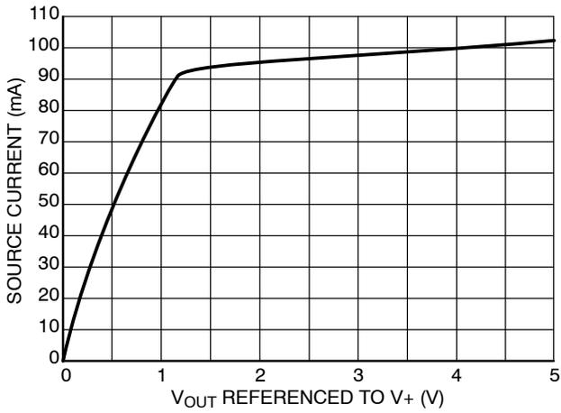
**Figure 19. Source Current vs. Output Voltage**
