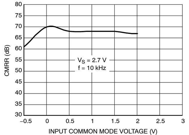
Figure 4. CMRR vs. Input Common Mode Voltage
