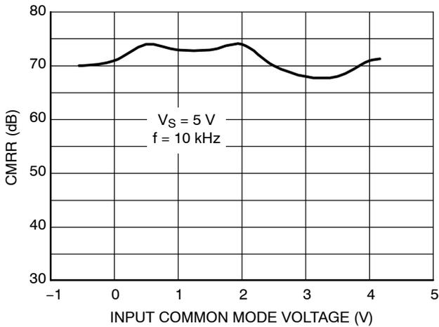
Figure 5. CMRR vs. Input Common Mode Voltage
