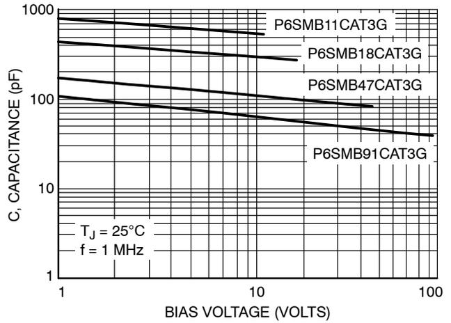
Figure 4. Typical Junction Capacitance vs. Bias Voltage
