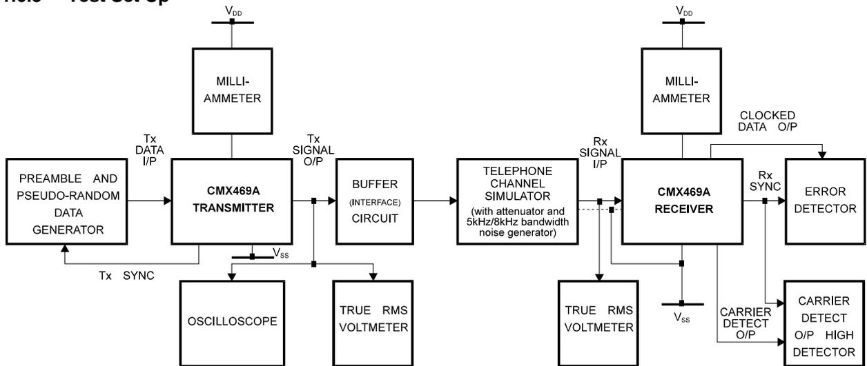
Figure 3 Suggested CMX469A Test Set-Up
