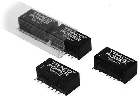
The TMR series is a range of miniature regulated 2 Watt DC/DC- converters in a SIL-package. Requiring only 2cm<sup>2</sup> board space they provide a state of art functionality. Wide 2:1 Input voltage range, 1000 VDC isolation voltage, external on/off control and a temperature range of -40°C – 75°C with no derating makes this converter suitable for many applications in telecommunication, control units and industrial equipments.
