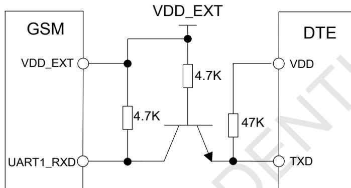
Figure 22: RX level matching circuit
