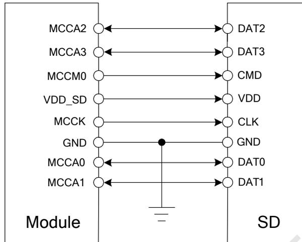
**Figure 34: SD reference circuit**
