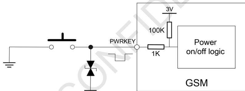
**Figure 14: Powered on/off GSM using button**
