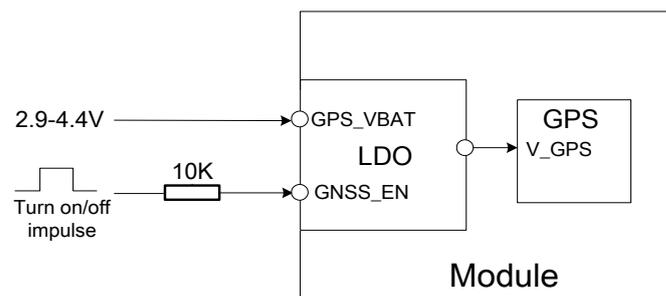
**Figure 43: Power on/off GNSS**
