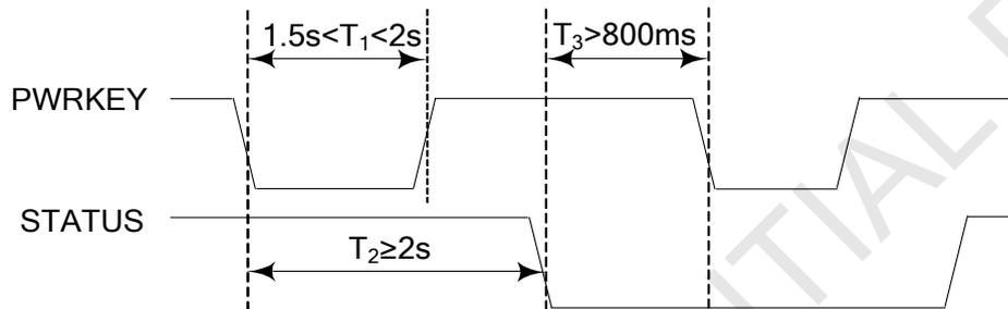
Figure 17: Timing of restart GSM
