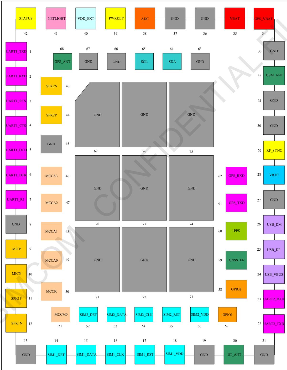
Figure 51: PIN assignment
