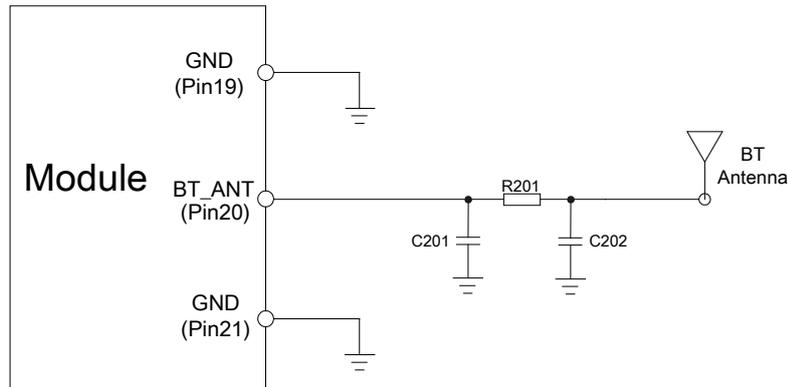
**Figure 39: Bluetooth antenna matching circuit**
