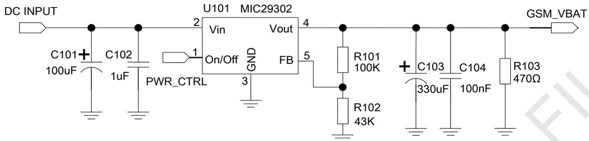
**Figure 10: Reference circuit of the LDO power supply**
