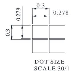
The non-specified tolerance of dimension is ±0.3mm.
